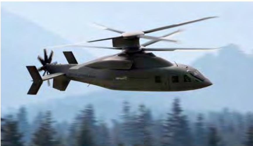
The Boeing-Sikorsky DEFIANT X compound helicopter features two co-axial rotors and a pusher propeller.
