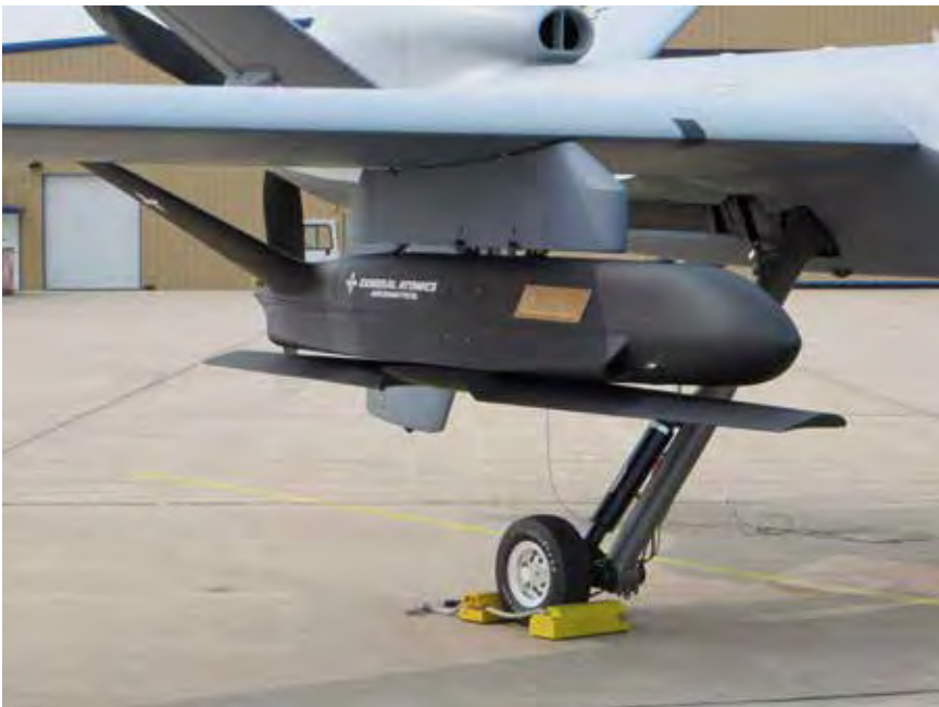
General Atomics Aeronautical Systems, Inc. (GA-ASI) conducted captive carry SPARROWHAWK Small Unmanned Aircraft Systems (sUAS) flight demonstrations in September 2020. The SPARROWHAWK aircraft is designed as an airborne launch and recovery demonstrator aircraft tailored to fit GA-ASI platforms, and is focused on Advanced Battle Management System’s technologies. It or similar small UAVs could be carried as payload aboard attritable aircraft.
