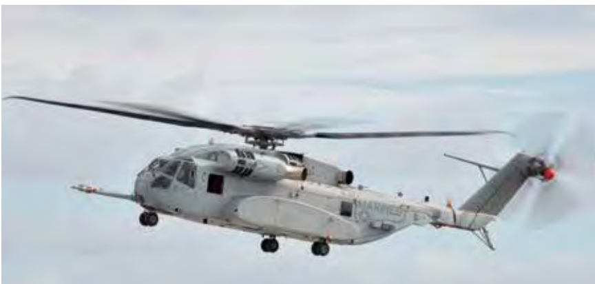
The CH-53K heavy lift helicopter features so many system upgrades and performance improvements over the predecessor CH-53E that it is frequently considered a de facto new aircraft. The lift capacity is nearly triple that of the baseline CH-53E.
