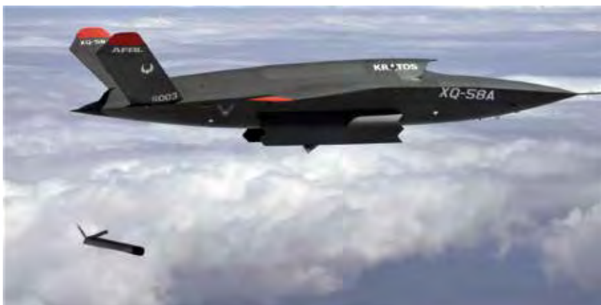
The XQ-58A VALKYRIE is designed for high speed and agile manoeuvrability. Depicted is a VALKYRIE deploying an ALTIUS 600.
