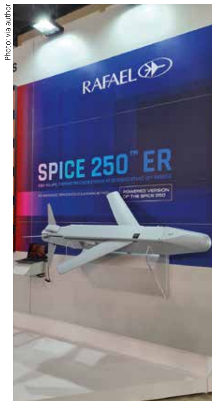
SPICE 250 uses inertial navigation and electro-optic scene-matching.
