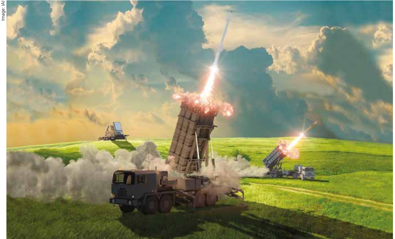
A variant of the STUNNER hit-to-kill missile; the highly advanced SkyCeptor interceptor is developed to defeat short- to medium-range ballistic and cruise missiles and other advanced air defence threats.
