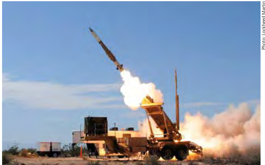
The Lockheed Martin Missiles & Fire Control PATRIOT PAC-3 MSE missile during live fire testing. The PAC-3 MSE is optimised for ballistic missile defence but retains capability against a range of targets from small UAS through manoeuvring fast jets.
