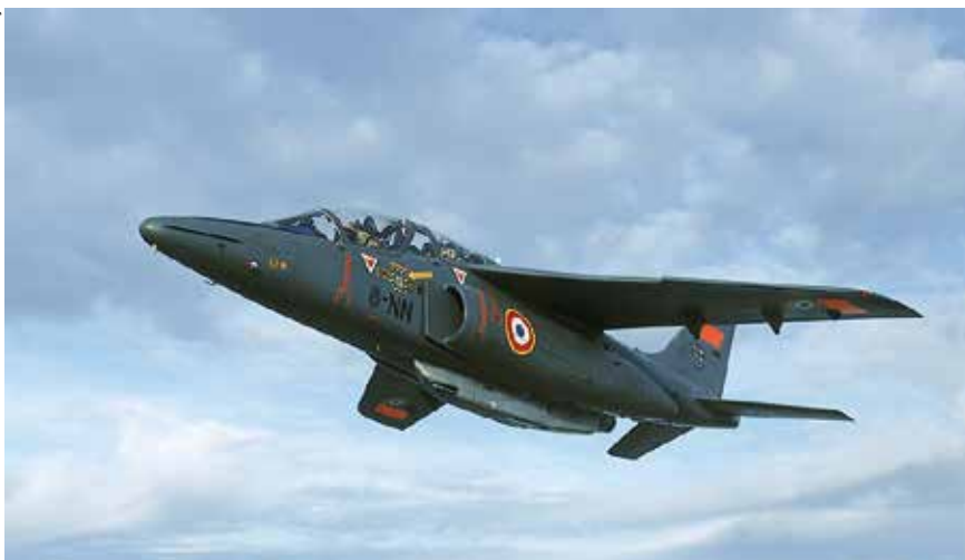
An ALPHA JET of the French Navy in flight. The ALPHA JET was developed to meet the advanced jet trainers needs of both France and Germany. Apart from its training mission, attack versions of the aircraft were developed to meet the requirements of export customers.
