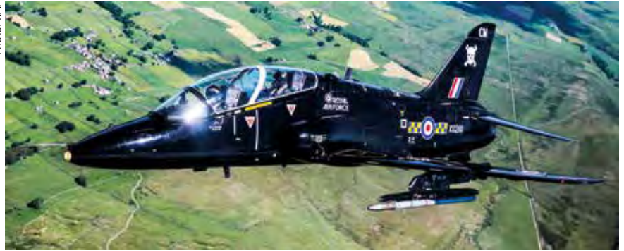
In 1972, the RAF placed an order for 175 HAWK T.1 advanced jet trainers. During the 1980s, numbers of these aircraft were upgraded to the T.1A configuration to act as a lightweight day fighter equipped with SIDEWINDER missiles and a gun pod.
