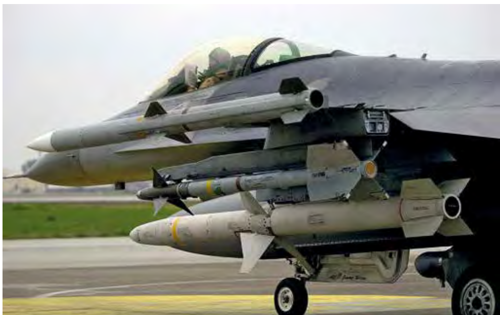
Standard SEAD capabilities include kinetic effects delivered by weapons like the Raytheon/Northrop Grumman AGM-88 High Speed Anti-Radiation Missile.
