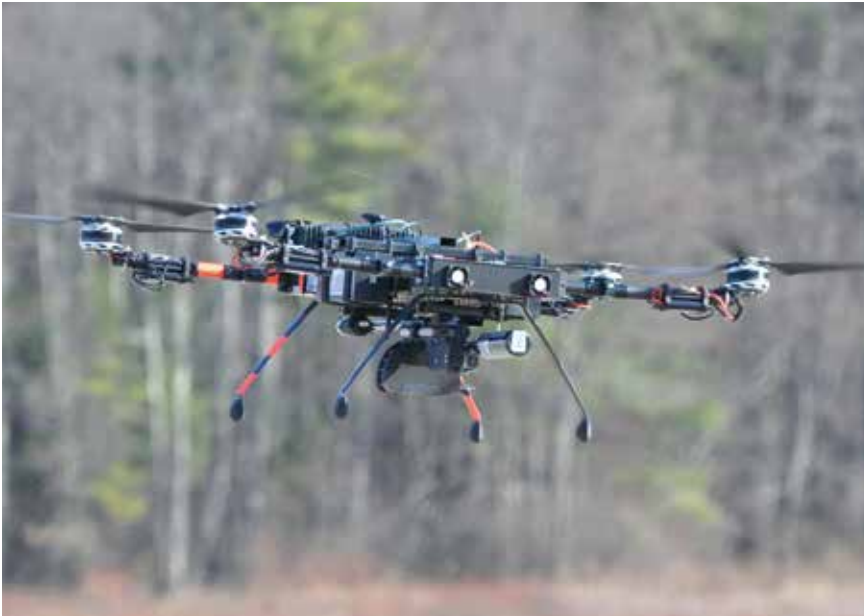
Aurora's Modular Intercept Drone Avionics Set (MIDAS) is an AI-enabled autonomous solution with optical sensors and a customised payload designed to defeat multiple adversarial UAS.
