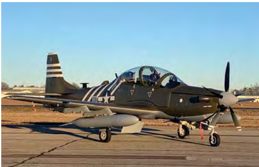
Embraer developed the original TUCANO as both a training aircraft and counter-insurgency aircraft. The latest A-29 SUPER TUCANO variant continues to offer both combat and training capabilities. The US acquired 20 SUPER TUCANO aircraft to give the Afghan Air Force a light attack capability.
