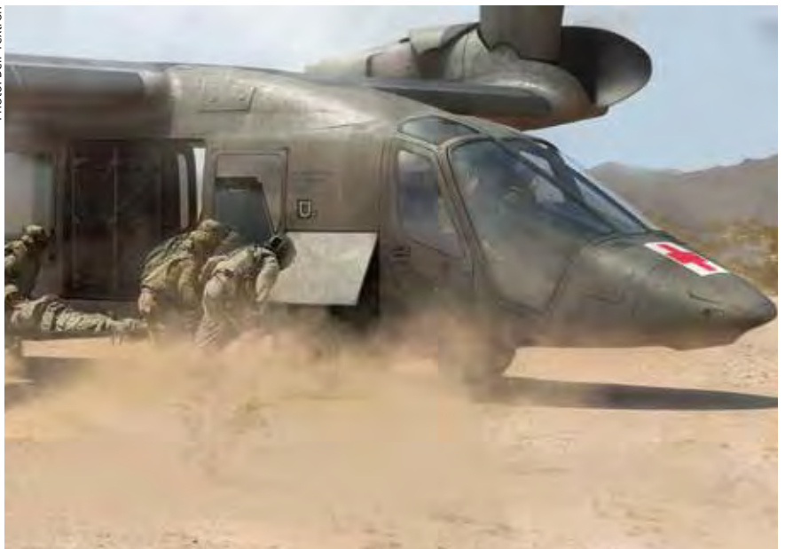
Concept of the Bell-Textron V-280 VALOR tiltrotor in the casevac role. The V-280 cruises at 280 knots and has a 500 nm operational range.
