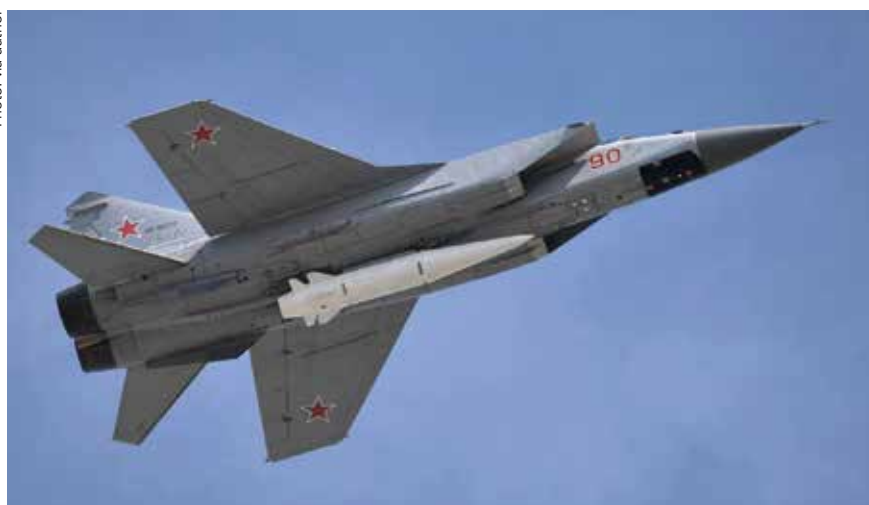
A MiG-31K carrying Russia's first operational air-launched land-attack hypersonic missile known as the Kh-47M2 KINZHAL
