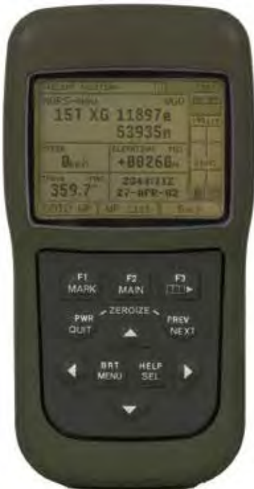
The DAGR is a mobile-held military GPS device that has appropriate encryption/coding and generates military coordinates.
