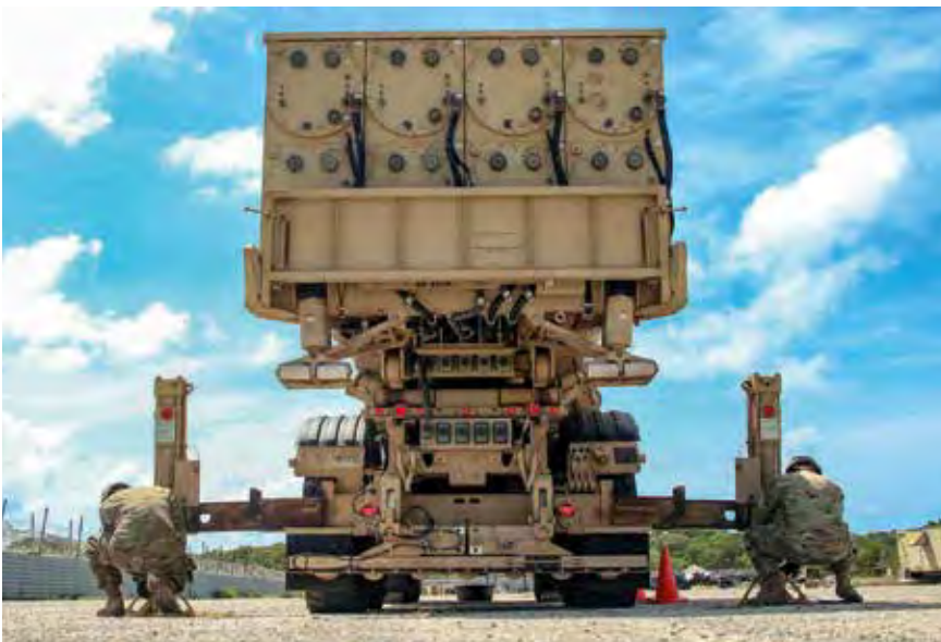
Soldiers train with a Terminal High Altitude Area Defence system for short- and medium-range missile defence at Andersen Air Force Base, Guam. A THAAD system was deployed briefly at the AEGIS ASHORE site at Deveselu Air Base in Romania in 2019 to enable the updates to the AEGIS system.
