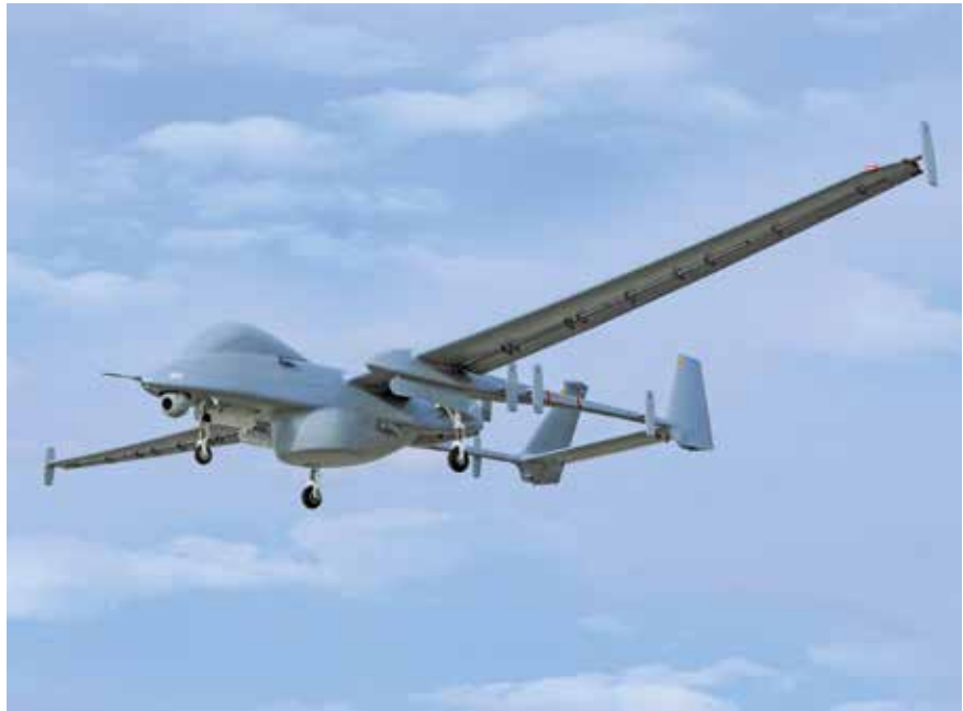
IAI's HERON family can fly in autonomous mode, though the aircraft are always monitored by human operators.
