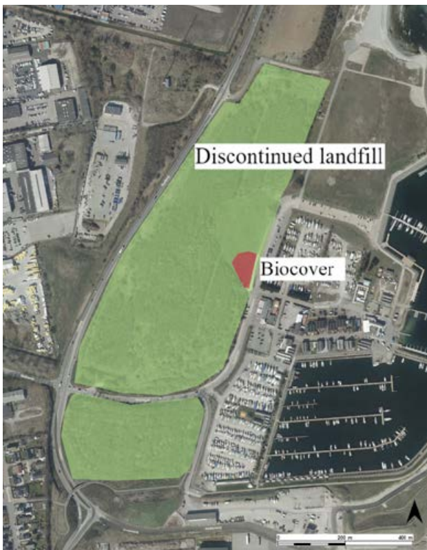
Figure 3.5 The discontinued Køge Landfill – “Tangmoseskoven” and the biocover. The biocover is shown in red.
