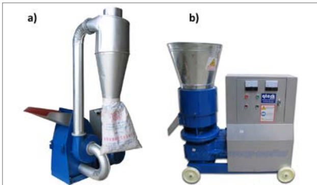
Figure 1.13 (a) Hammer Mill HM 426, (b) pelletizing machine PP295UG-S (picture source: https://www.qteck.de/ )
