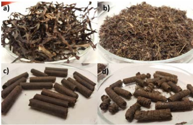
Figure 1.12 (a) raw eelgrass, (b) shredded eelgrass, (c) eelgrass pellets, (d) eelgrass pellets with added water
