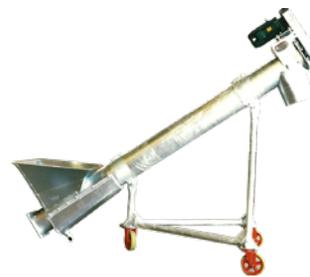
TRANSPORTADOR CON ALTURA FIJA Y RUEDAS PARA MOVILIZARLO
