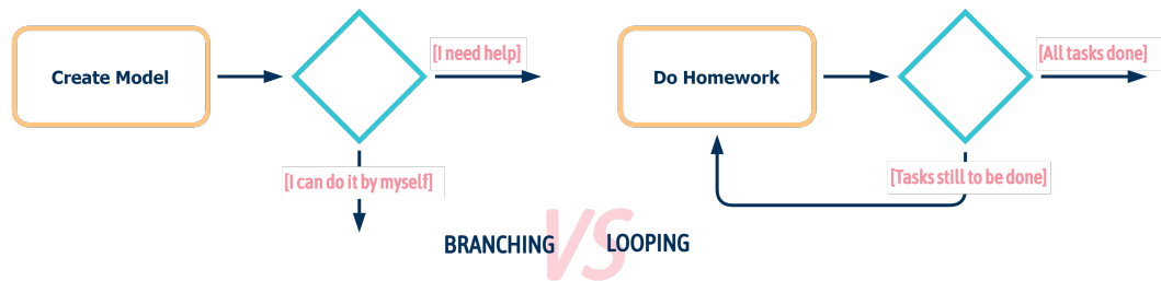
Figure 2.5: Conditional Branching v. Looping in an Activity Diagram
