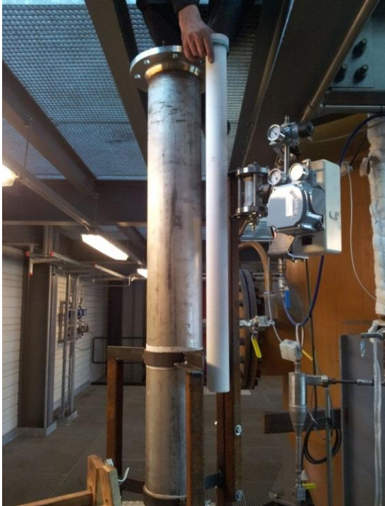
Figure 47: Filter element (right) and filter-house (left).
