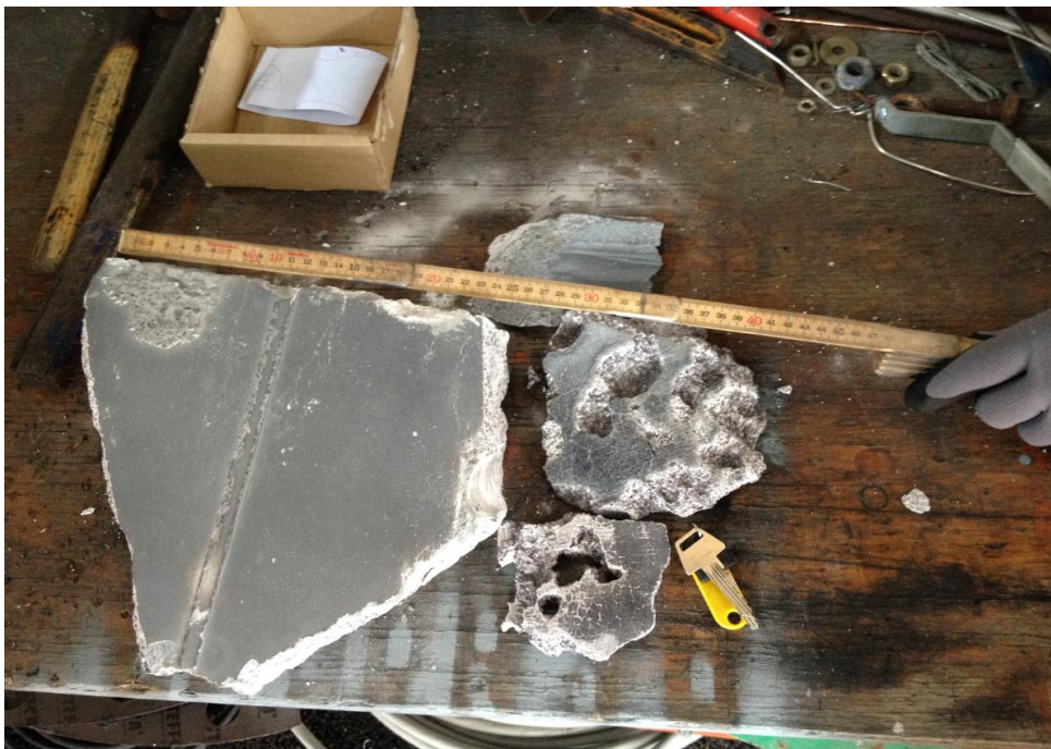
Figure 30: Piece of refractory in the CR bed
