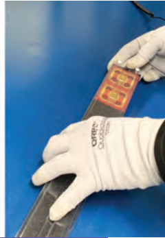
ESD precautions include ionizers, gloves and wrist straps
