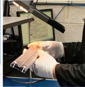
ESD precautions include ionizers, gloves and wrist straps
