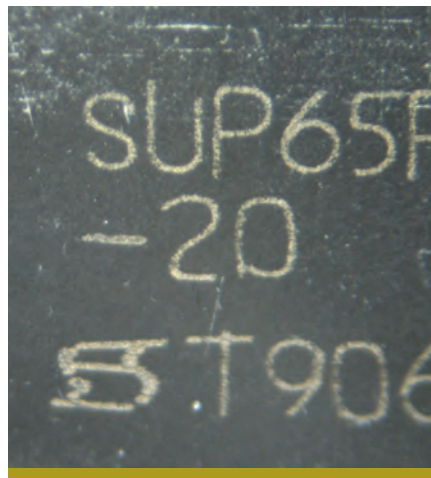
This sloppily labelled part features an out of proportion Siliconix logo
