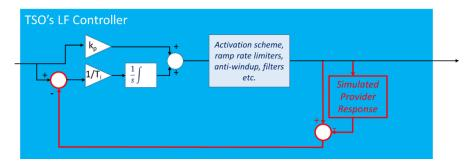
Figure 17: Simplified scheme that feeds back the expected response of aFRR providers
