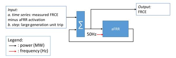
Figure 37: High level Matlab/Simulink model of the individual LFC Blocks in the CE system
