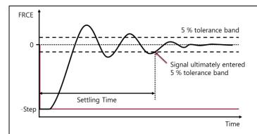
Figure 14: Calculation of settling time
