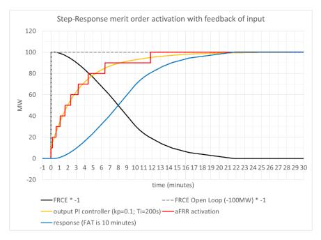
Figure 18: Step response for 100MW step of merit-order activation scheme with a feedback loop (to be compared with Figure 11)  $^{12, 17}$ .
