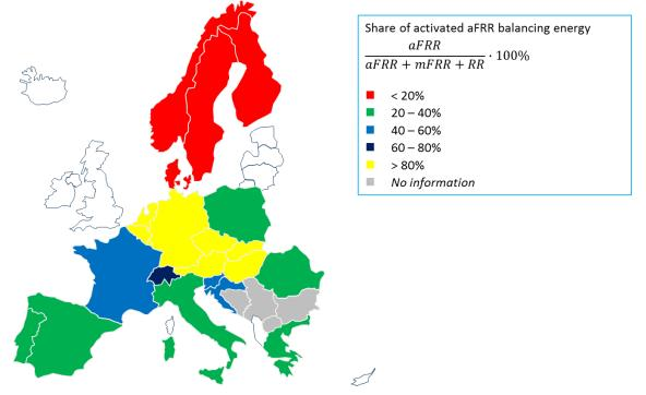
Figure 2: Share of aFRR energy in total activated FRR/RR balancing energy, based on figures for February and June 2015<sup>9</sup>.
