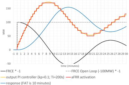
Figure 11: Small deviation (100MW step response) for pro-rata (upper figure) and merit-order (lower figure) activation scheme (300MW of aFRR connected to the LFC)<sup>12, 17</sup>.
