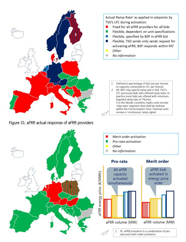
Figure 32: TSOs that apply a pro-rata activation scheme or a merit-order activation scheme
