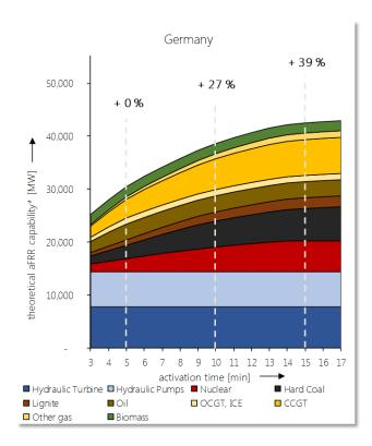
Figure 20: Example of a theoretical aFRR capability diagram for Germany (percentages are the change from current FAT) \* Upward and downward, not symmetric
