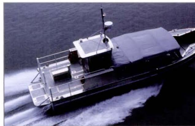
jet propulsion, is capable of speeds in excess of 25 knots over a 300nm range in sea state 2-plus. A bow ramp facilitates embarking and discharging personnel over a ramp, low pier, or quay.
