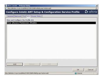
18. The **Power Policy** tab has configuration options to select the sleep states for Intel AMT and an **Idle Timeout** setting. It is recommended that Idle timeout is always set to **1** for optimal performance.
