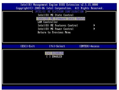
To assist with the manufacturing process as well as OEM-specific in-field firmware update processes, ME firmware provides an OEM- configurable capability that leaves the local firmware update channel always open no matter what value you select for the **ME Firmware Local Update** option.
