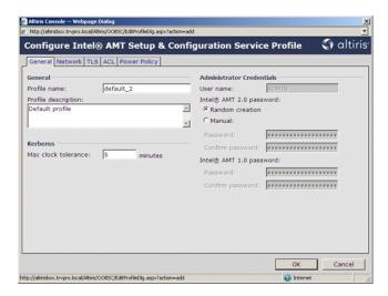
15. The **Network** tab provides the option to enable ping responses, VLAN, WebUI, Serial over LAN, and IDE Redirection. If you are configuring Intel AMT manually, all these settings are also available in the MEBx.
