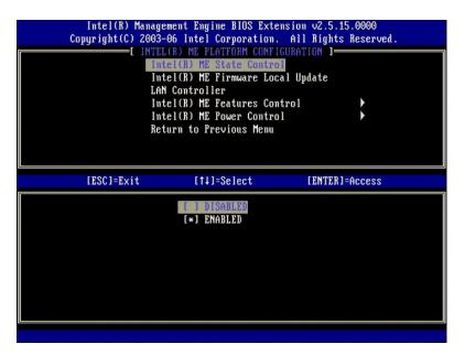
When enabled, the **ME State Control** option lets you disable ME to isolate the ME computer from the main platform while debugging a field malfunction. The table below illustrates the details of the options.
