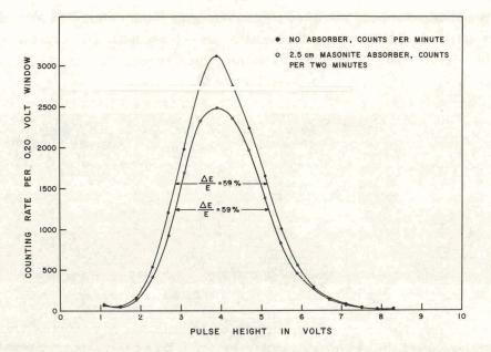
Figure 6. Differential pulse height spectrum of iodine-125. Pulse height vs. counting rate.
