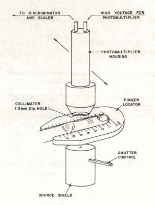
Figure 4. Diagram illustrating the position of finger locator, radiation source, collimator and photomultiplier.
