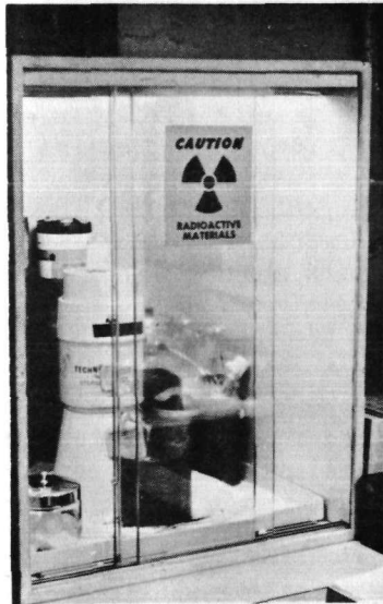
Figure 1. Mo-Tc house built of plywood, Pb lined epoxy painted, fluorescent light and 3 Pb glass doors. Base made as a tray to contain spills.
