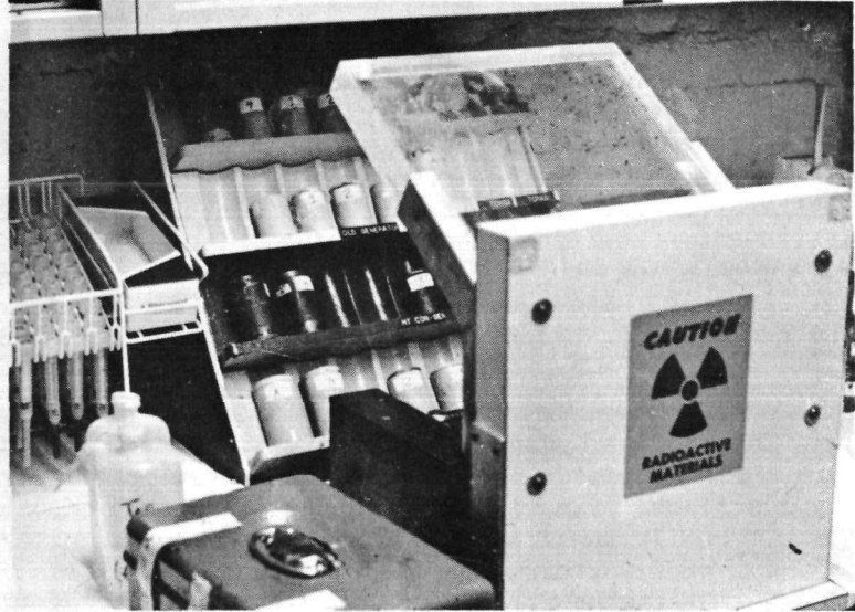
Figure 2. Eluate organizer rack for ^{99m}\text{Tc} placed immediately behind a face and body shield. Most radiopharmaceutical doses are prepared at this work station.
