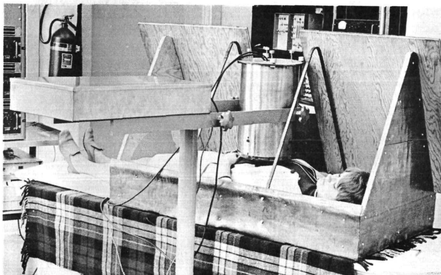
Fig. 2 Detector, counterbalanced stand and lead tent with near-side panels removed.
