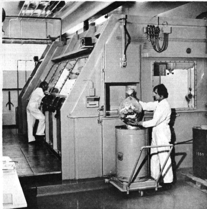
Fig. 2 : Exterior of the sorting box and the transfer box. An operator is loading a plastic bag into the sorting box, where another operator is sorting the waste from the conveyor belt into several drums or the press box (left background). The lower, closed sash door is used for the transfer of drums into the operations box, visible through the window at the right. \gamma -dose rate monitors are mounted at the working face of the boxes.
