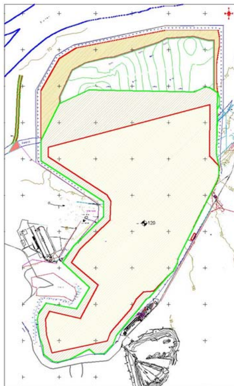
Figure 12 Final contour of the opencast mine Drmno with the inner dump in 2054
