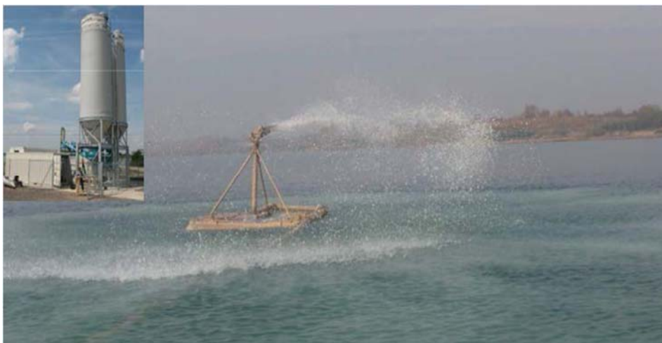
Figure 2 Upper left: Lake Hain stationary neutralisation plant and its floating unit for above water distribution (source: UIT/LMBV)
