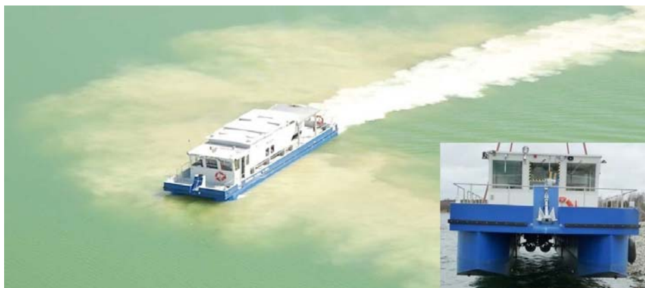
Figure 3 Water treatment vessel "Barbara" in operation, and (bottom right) being lowered – showing the distribution system between the vessel's hulls (source: LUG/LMBV)
