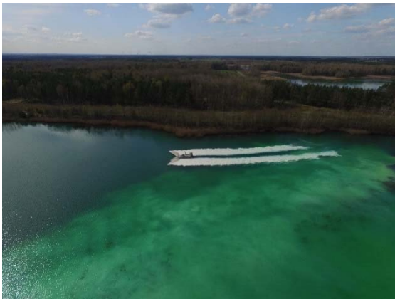
Figure 7 Aerial photo showing the distribution of chalk lime above the surface, lake Tröbitz 08.04.2016
