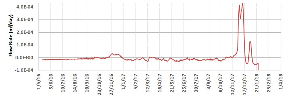
Figure 7 Flow rate at the surface between S&R and trafficability layers
