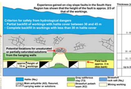
Figure 15 Hydrological danger due to solution streaming to the hanging wall
