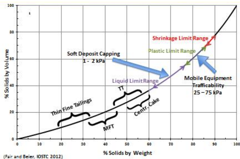
Figure 5 Fluid fine tailings FFT dewatering processes for oil sands tailings
