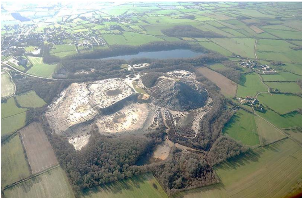
Figure 1 Aerial view of the site (tailings (left) and waste rocks (right) deposits, water-filled open pit)
