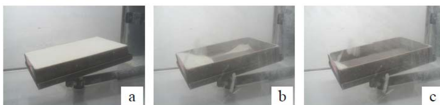
Figure 2 Wind tunnel test of tailing sands without treatment. (a) Time 0 (b) 5 min after applying wind at a speed of 12 m/s; (c) 20 min after applying wind at a speed of 12 m/s.
