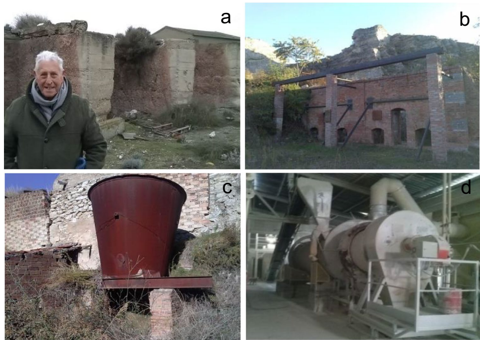
Fig. 8 Abandoned historic kilns: a type C located in Tauste (Zaragoza), b type E located in San Esteban (Huesca), c type F located in Albelda (Huesca), and d operating cylindrical rotary kiln (type G) located in Cuarte de Huerva (Zaragoza)
