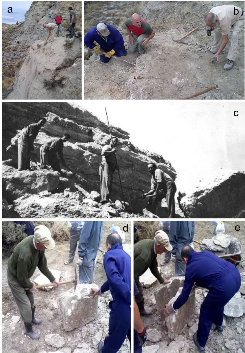
Fig. 5 Gypsum extraction: a removal of powdery gypsum in Navarrete (Teruel); b extraction of a gypsum block using a large gimlet, pick, and wedges; c historic photograph showing surface mining of gypsum in 1940 using picks and a digging bar in a family-owned quarry in San Esteban de Litera (Huesca) (photo courtesy of the “Centro de Estudios Literanos” in Huesca); d and e separation of a large gypsum block along the plane generated by the lamellar structure of the rock using a pick
