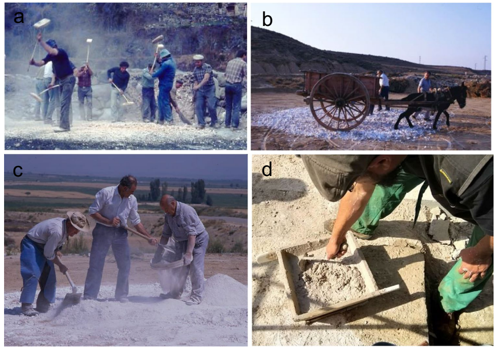
Fig. 11 Gypsum processing: a crushing of gypsum using the traditional “algadera” (Lanaja (Huesca) photo courtesy of E. Monesma Monge); b gypsum crushing using a cart (San Juan de Plan (Huesca) in 1981 (photo courtesy of E. Monesma Monge)); c traditional sieving of gypsum, and d kneading of gypsum using a wooden “bacía,” which was also used as a measuring unit
