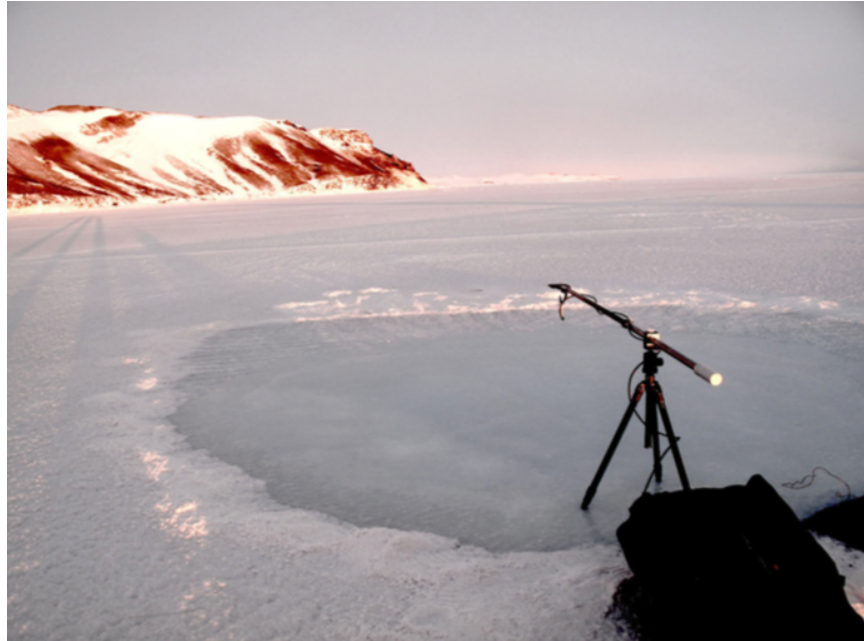
Sea ice in McMurdo Sound. Note area of bare sea ice cleared of 3 mm crust of salty snow. Instrument shown is an ASD radiometer to take spectral albedo measures. September 2009. Photograph courtesy of Regina Carns, reprinted from Carns et al. 2015.
