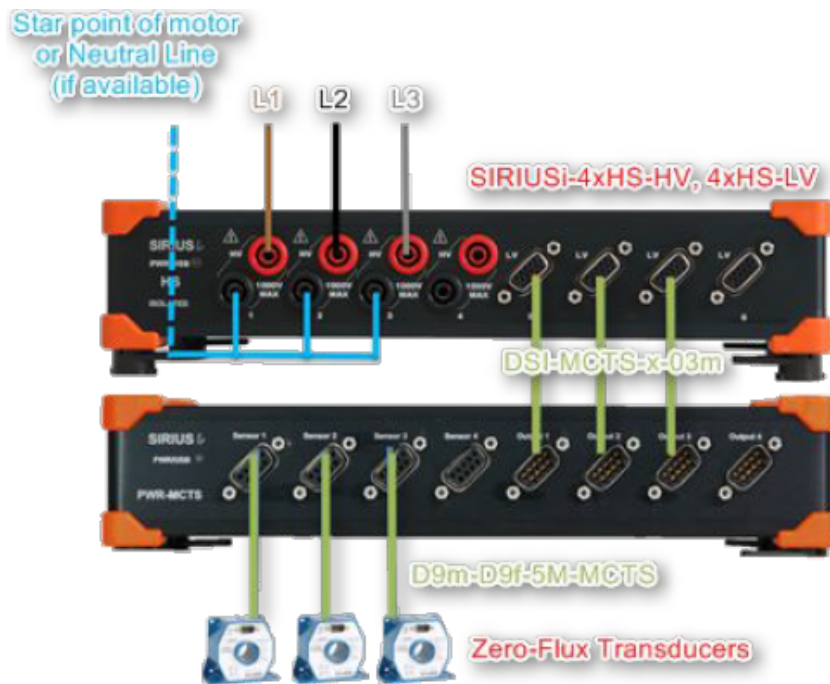
Three-phase system in star connection
