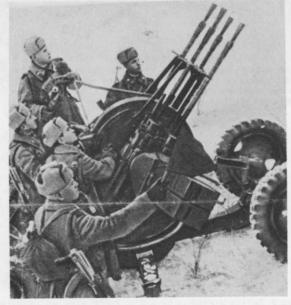
SOVIET 14.5-MM QUAD AA MACHINE GUN, ZPU-4.
