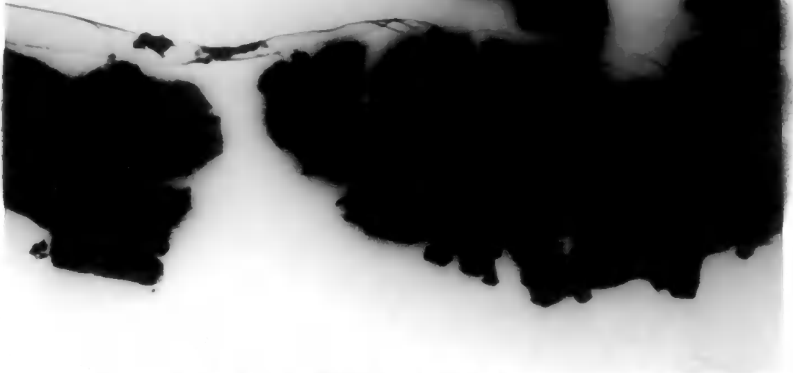
Plate 3.25 Calcium nitride hydrolyzed with steam at 120° for 30 min. \times 15,000
