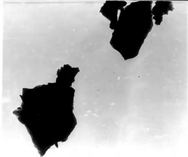
Plate 6.3 Titanium nitride calcined at 1000° for 20h. x 15,000
