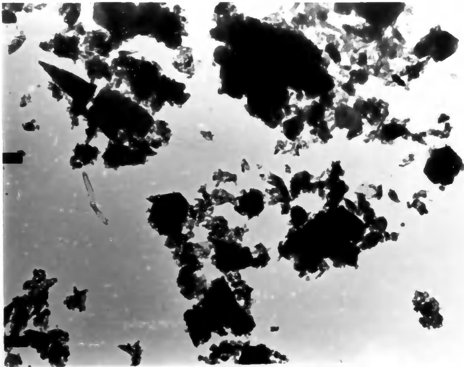
PLATE 3.16 Calcium nitride, wet, hydrolyzed at 22° for 24 hr. x 15,000
