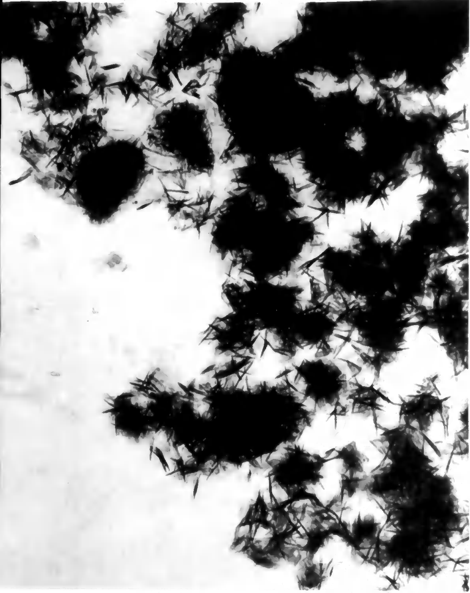
1/4 Photo 2.30 Magnecium oxide 'wet' hydrated at 22° for 2h. x 15,000
