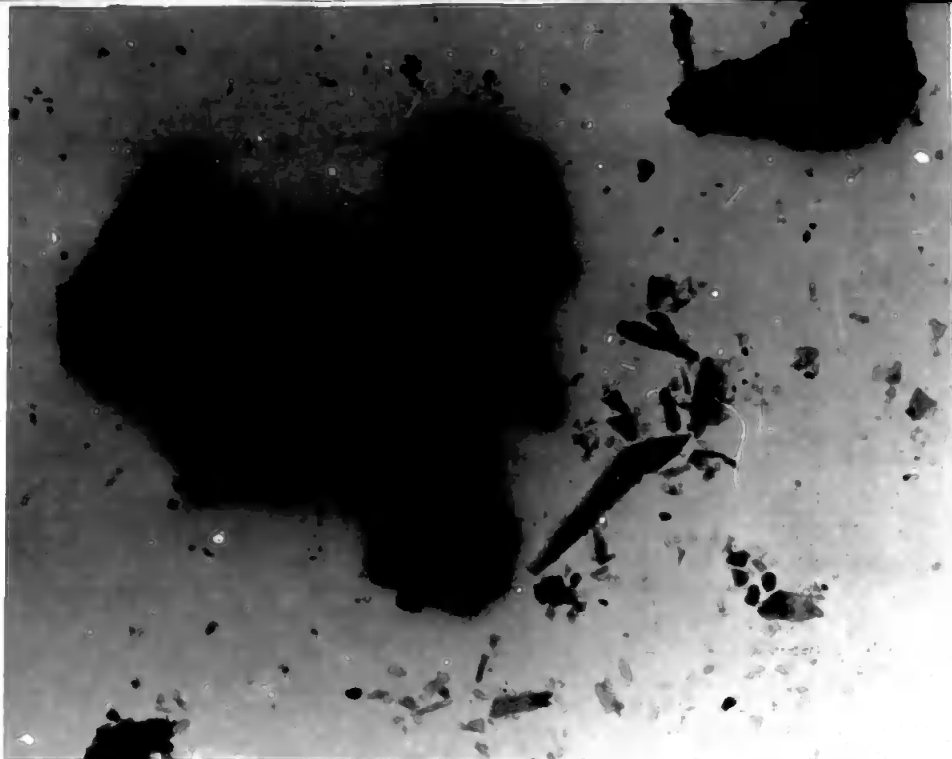
Plate 3.20 Precipitated calcium hydroxide x 15,000
