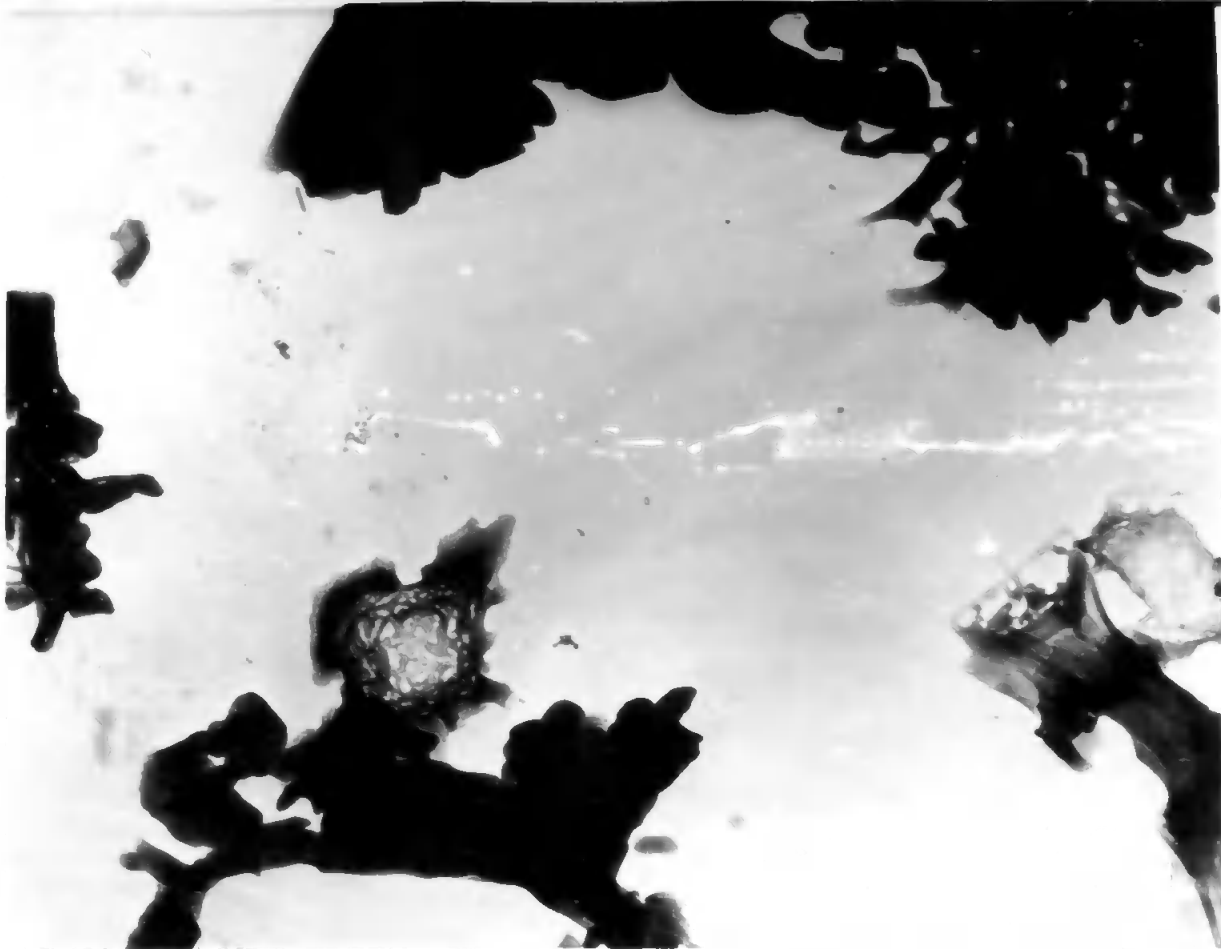
Plate 9.7 Baron nitride calcined for 6 days at 500° x 15,000
