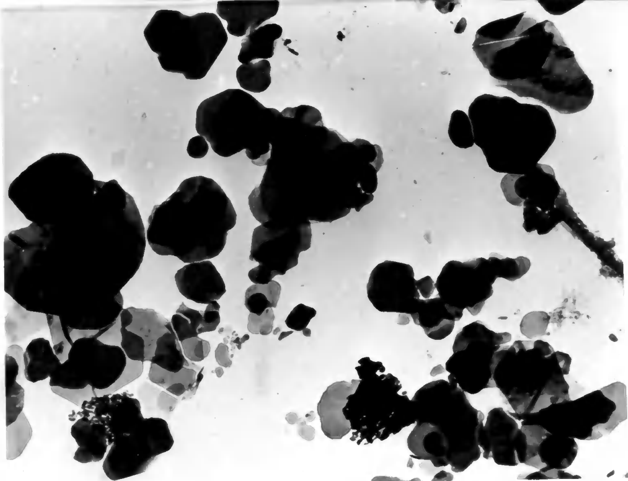
Plate 3.3 Barium nitride calcined at 450^{\circ} for 24h. \times 15,000
