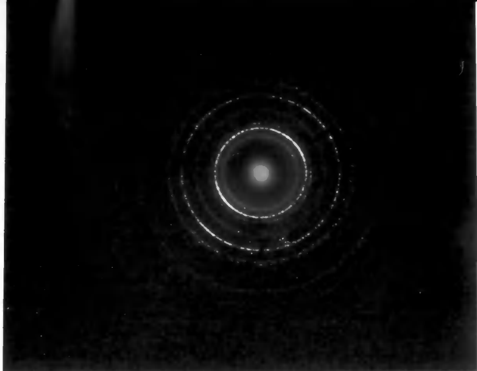
Plates 4.2 (above) and 4.4 (below) Electron diffraction patterns of zinc film before and after heating in ammonia (cf. Plates 4.1 and 4.3)
