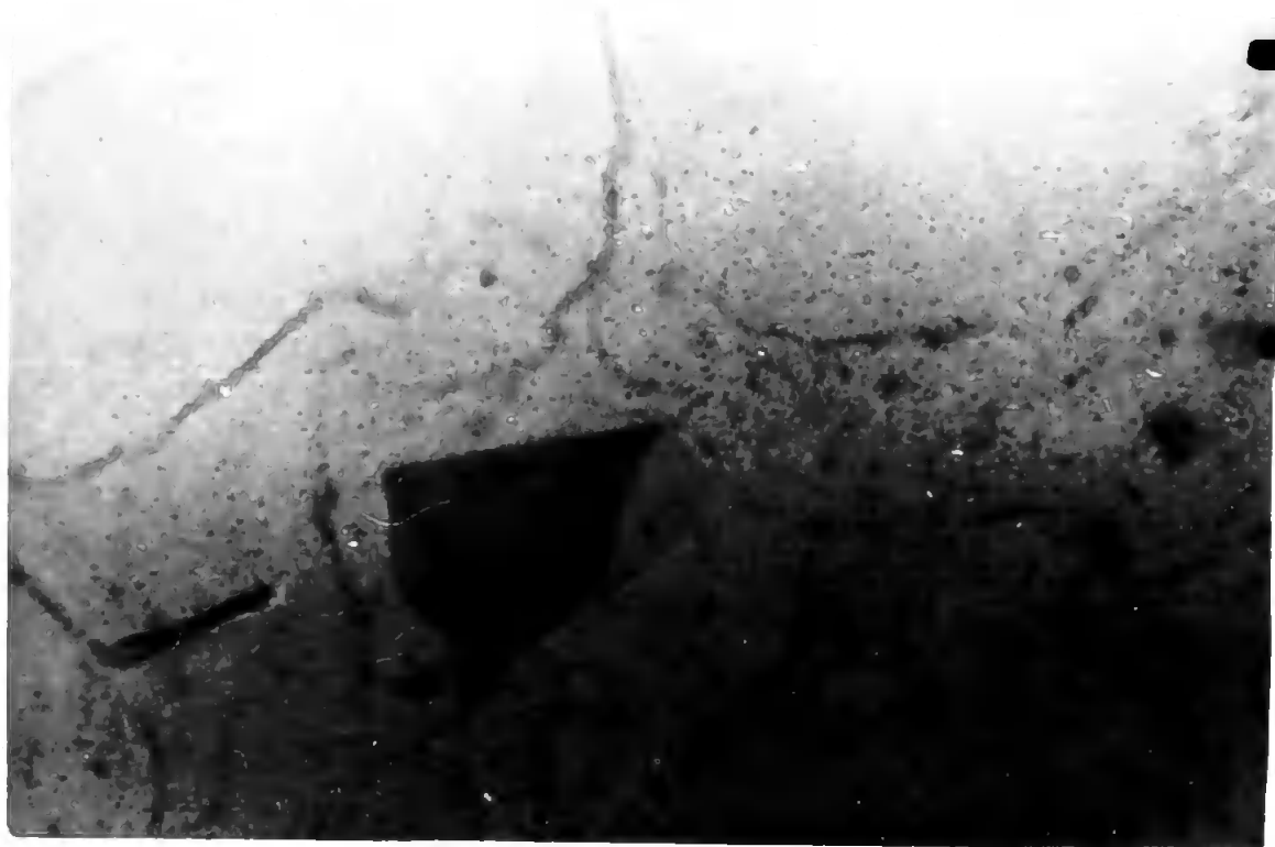
Plate 3.3 Less uniform, vapour deposited magnesium film x 15,000
