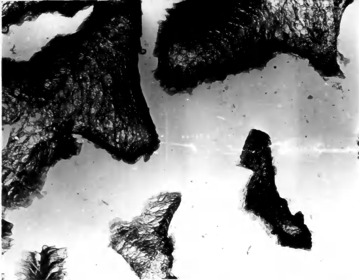
Plate 9.3 Boron nitride calcined at 900° for 6 days x 15,000
