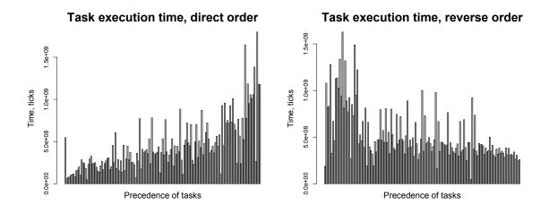
*Figure 5.29: Distribution of tasks in a Jacobi sum program. Left: without a task pool transformation. Right: with said transformation.*
