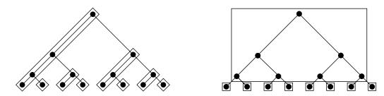
*Figure 6.3:* Divide and conquer expansion schemes binary trees, depth 3. Left: distributed expansion, right: flat expansion. Boxes symbolise processes.
