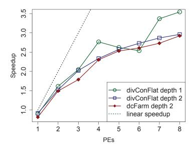
Figure 6.39: Comparing the speedups for divConFlat and dcFarm on sakania.
