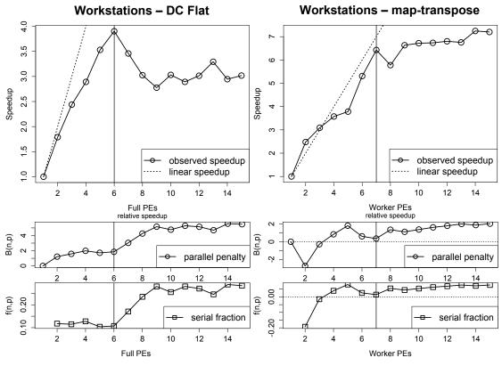
Figure 6.22: Evaluation of FFT on local workstations.
