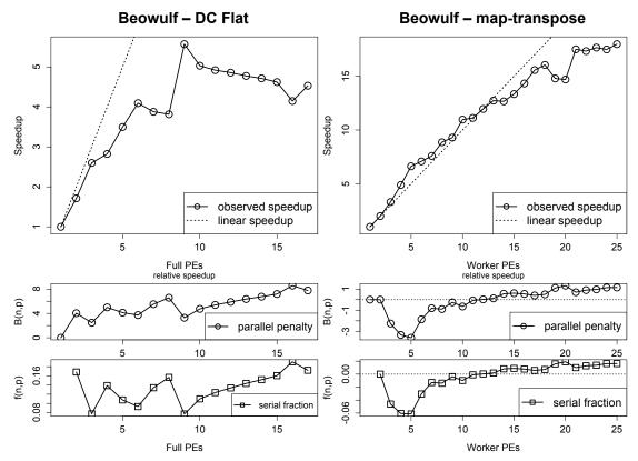
Figure 6.23: Evaluation of FFT on Beowulf cluster.
