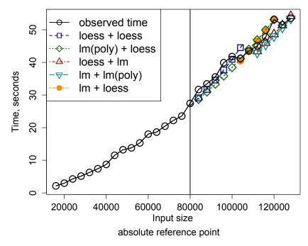
*Figure 6.15: Predicting the parallel execution time of Karatsuba multiplication.*
