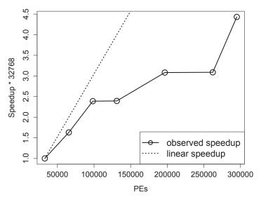
Figure 4.3: The speedup plot for LBM.
