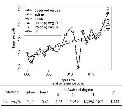
Figure 5.34: Predicting sequential execution time of Jacobi sum test.
