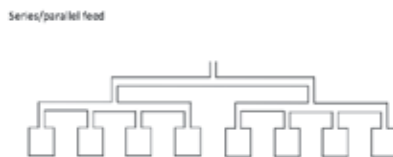
Fig. 5. Series-Parallel feed configuration for microstrip arrays. After (Lee, 1997)
