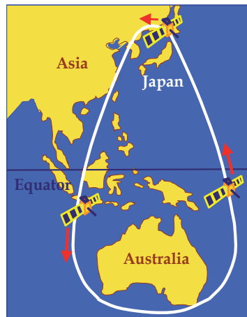
Fig. 43. Apparent orbits of three planned 24-hour QZSS-satellites with inclination i = 42.5^\circ and eccentricity e = 0.21 .
