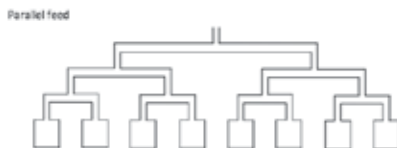
Fig. 4. Parallel feed configuration for microstrip arrays. After (Lee, 1997)
