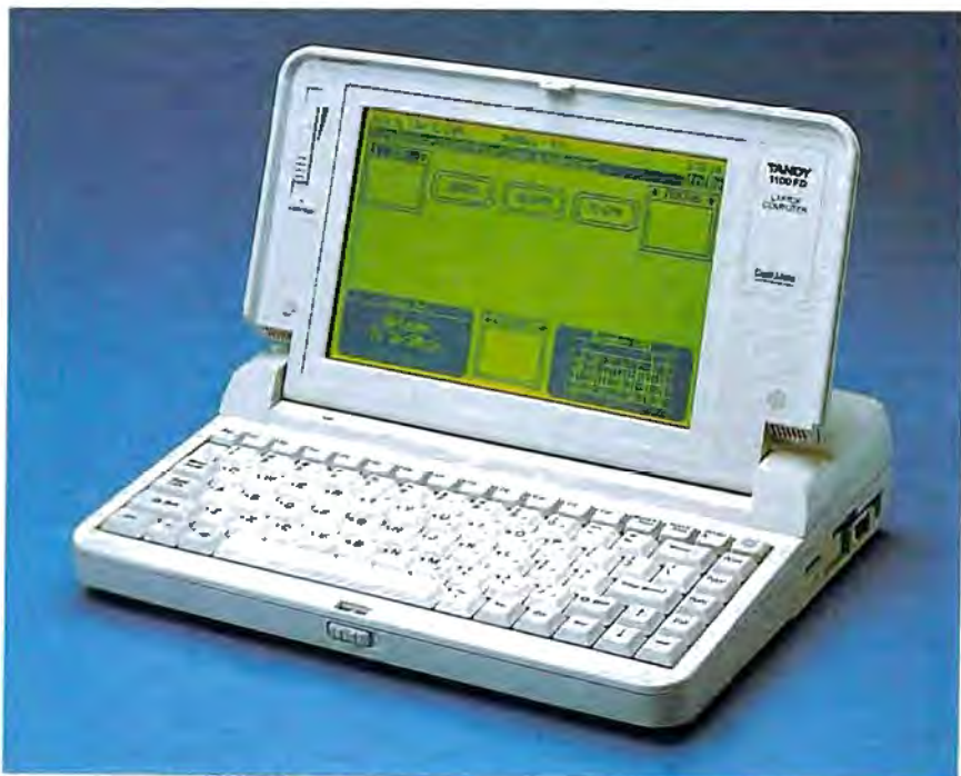
The lightweight Tandy 1100 FD laptop computer sports a nonbacklit green LCD display and a single 720K floppy drive, and it carries the DeskMate graphical interface in ROM.
