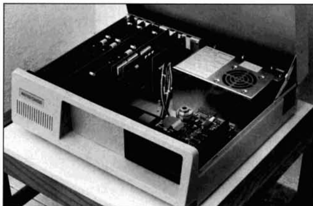
Master/Chassis lets you plug in eight IBM-size boards and add one to four half-height drives.
