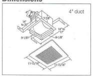
Whole-House (60 CFM) and Spot (110 CFM) ventilation combined in a 2-speed ceiling mount fan.
