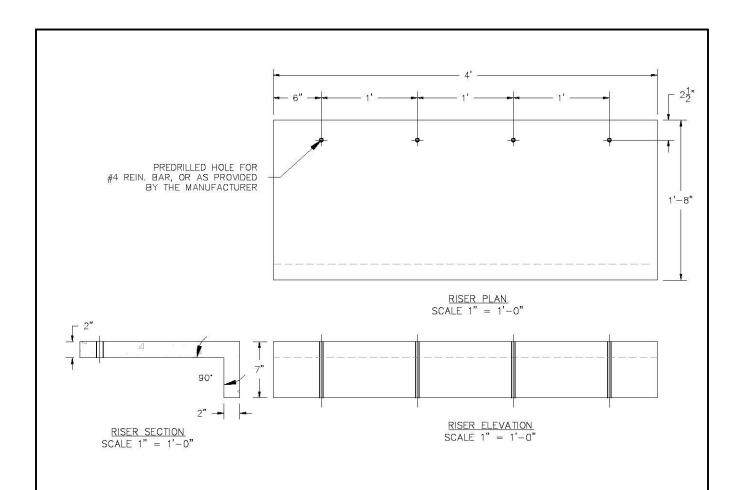
NOTES: A. RECOMMENDED SUPPLIER: PACIFIC CONCRETE INDUSTRIES, 360-734-0910, OR APPROVED EQUAL. B. SEE DETAILS 03300.01, 03300.02, 03300.04 FOR PLACEMENT DETAILS.
