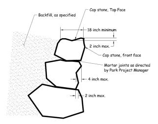
Figure 1 - Rock Wall Partial Section View
