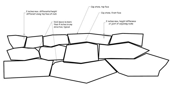
Figure 2 - Front Face Partial Elevation View
