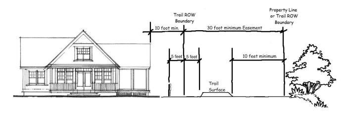
Figure 1 - Example of Minimum Trail Setbacks from Buildings, Other Structures, and Property Lines
