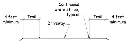
Figure 2 - Paved trail with no buffer
