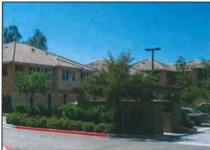
3.2.2.7a) Trash enclosures with landscape screens and architecture that is similar to that of the project help to minimize the negative visual impact of these structures.
