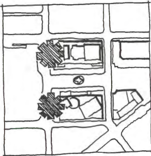
13. To preserve the Fulton Street view corridor, no parking or bus staging is permitted in the mall area. The vehicular drop off should be flexible and as small as possible. White zones and bus drop off should be located along Larkin Street.
