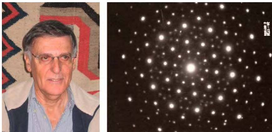
Figure 1-14. Dan Shechtman (photograph by the authors) and his electron diffraction pattern with 10-fold symmetry (photograph courtesy of Dan Shechtman, Haifa).
