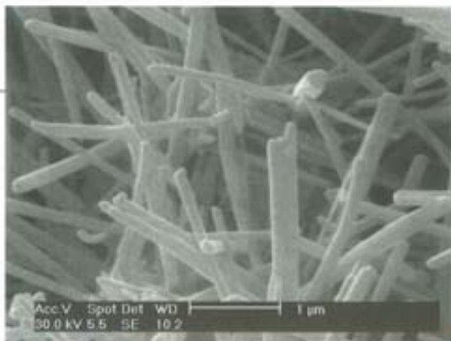
Electron microscope photo (SEM) 20,000x Cement paste with a high water/cement ratio Note the spaces between the "needles" of C-S-H that result in low mechanical strength
