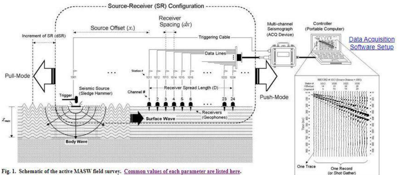
Fig. 1. Schematic of the active MASW field survey. [Common values of each parameter are listed here.](#)
