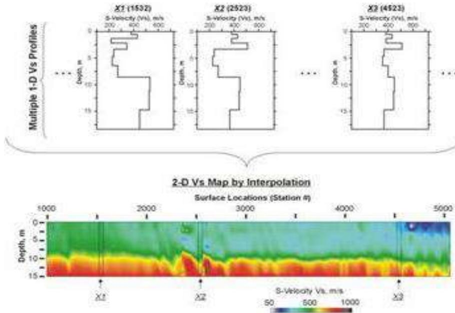
**Figura 10:** Procedimiento global de velocidades de ondas S. Fuente: Kansas Geological Survey [www.kgs.lu.edu/software/surfseis](http://www.kgs.lu.edu/software/surfseis) [www.masw.com/Vs2DInversion.html](http://www.masw.com/Vs2DInversion.html)
