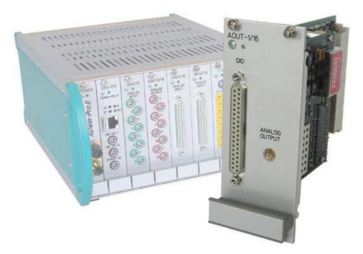
These ADwin-PRO-II systems are desktop units featuring a ½ 19" enclosure (9-inch wide, 5 ¼ inch high), a 10-35V DC-DC converter and 7 data acquisition card slots. All modules are mounted from the front side. The ADwin **PRO-II T11 processor module** features the **ADSP TigerSharc © processor** with 300 MHz clock speed, 768 MB internal memory and 256 MB of RAM. The T11 processor has extremely short response
