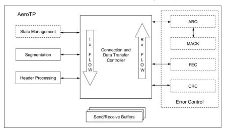
Figure 4. AeroTP implementation architecture
