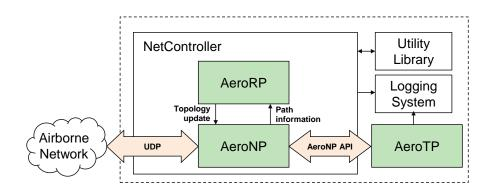
Figure 3. System Architecture
