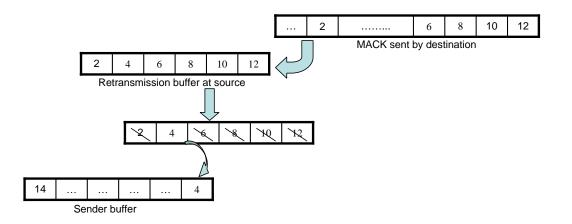
Figure 7. AeroTP ARQ retransmission mechanism
