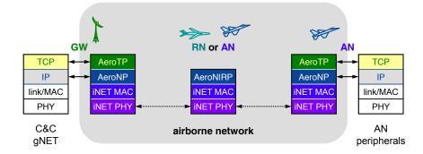
Figure 2. Airborne network protocol architecture
