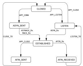
Figure 8. AeroTP state machine
