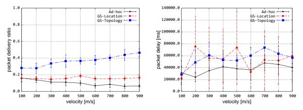
Figure 13. Effect of node velocity on PDR
