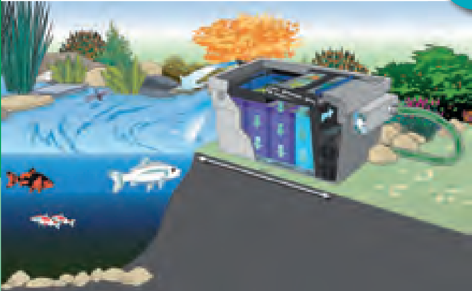
Schematic diagram: UVC clarifier in combination with OASE BioTec ScreenMatic 2 flow-through filter
