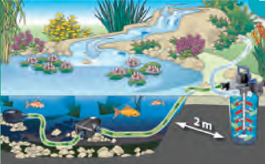
Schematic diagram: Pressure filter FiltoClear in combination with filter and watercourse pump
