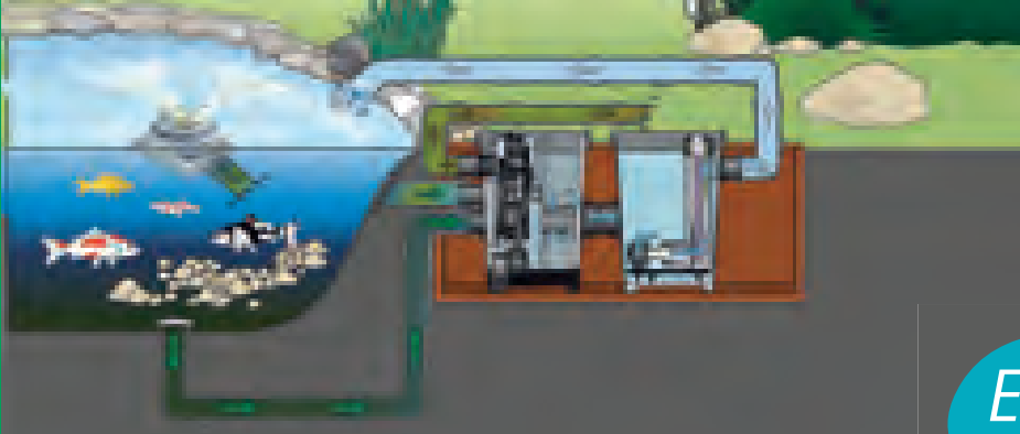
Schematic diagram: ProfiClear Premium Compact gravity-fed
