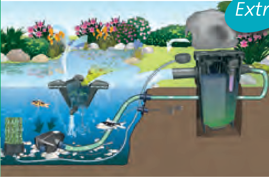
Schematic diagram: Interaction of the functions in the Clear Water System
