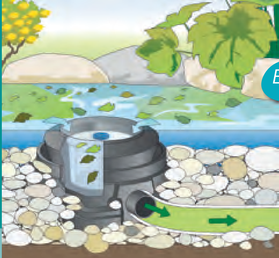
Schematic diagram: ProfiSkim 100 in use
