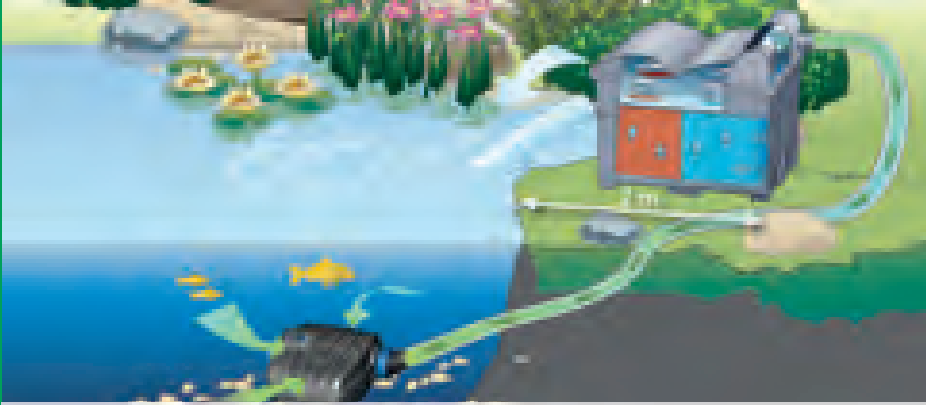
Schematic diagram: BioSmart UVC 16000 in combination with filter and watercourse pump AquaMax Eco Classic
