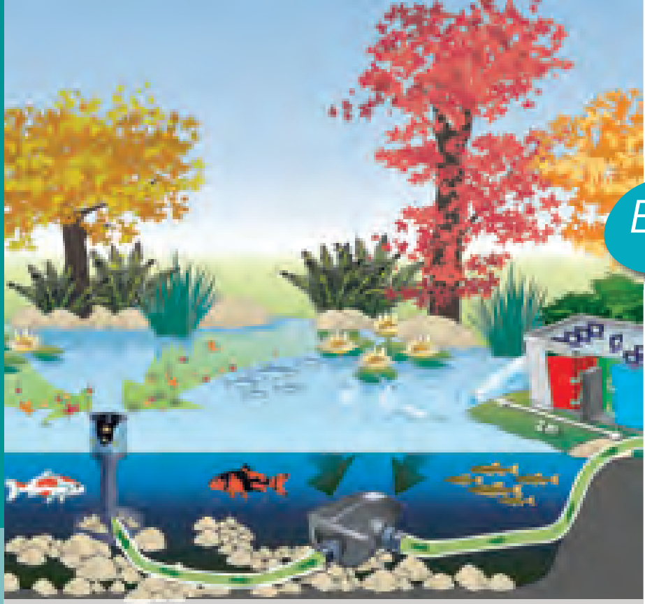
Schematic diagram: AquaSkim in use with filter and watercourse pump AquaMax Eco Premium
