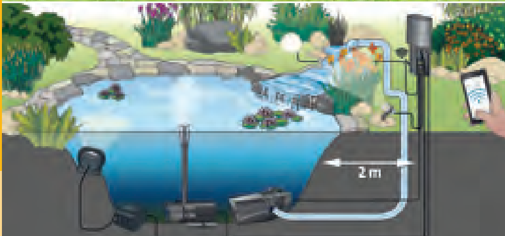
Schematic diagram: Connection possibilities with the OASE garden power outlet InScenio FM-Master WLAN
