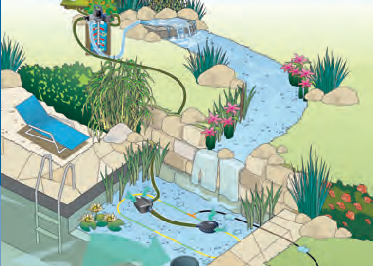
Schematic diagram: Filter and watercourse pump AquaMax Eco Premium 12 V (PRO) used in the swim pond in combination with an OASE pressure filter FiltoClear (PRO)
