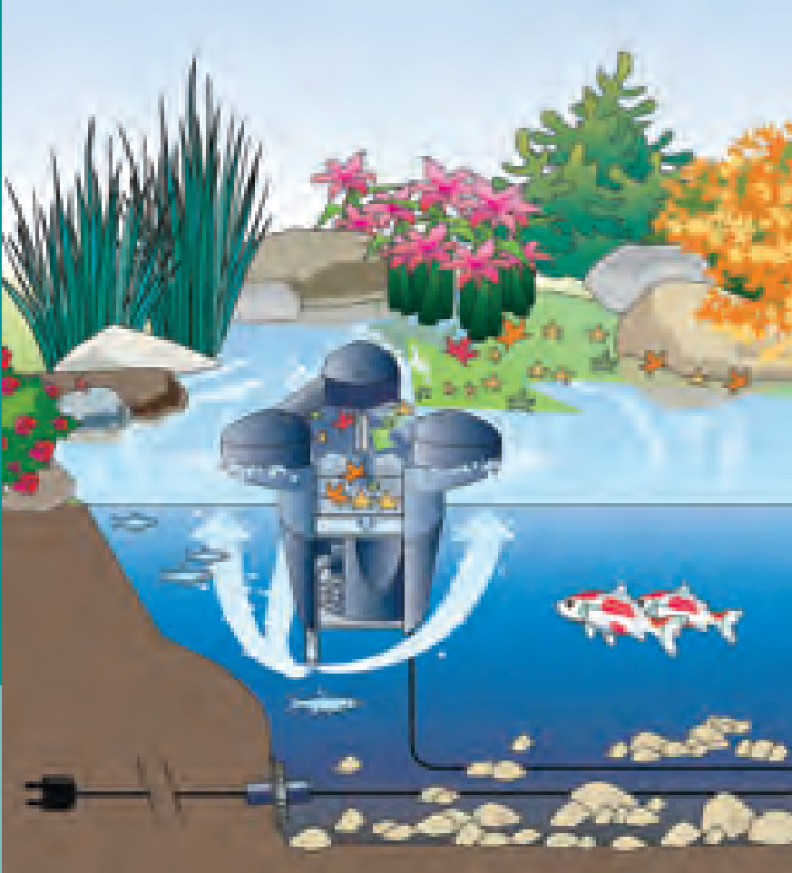
Schematic diagram: SwimSkim 25 in use
