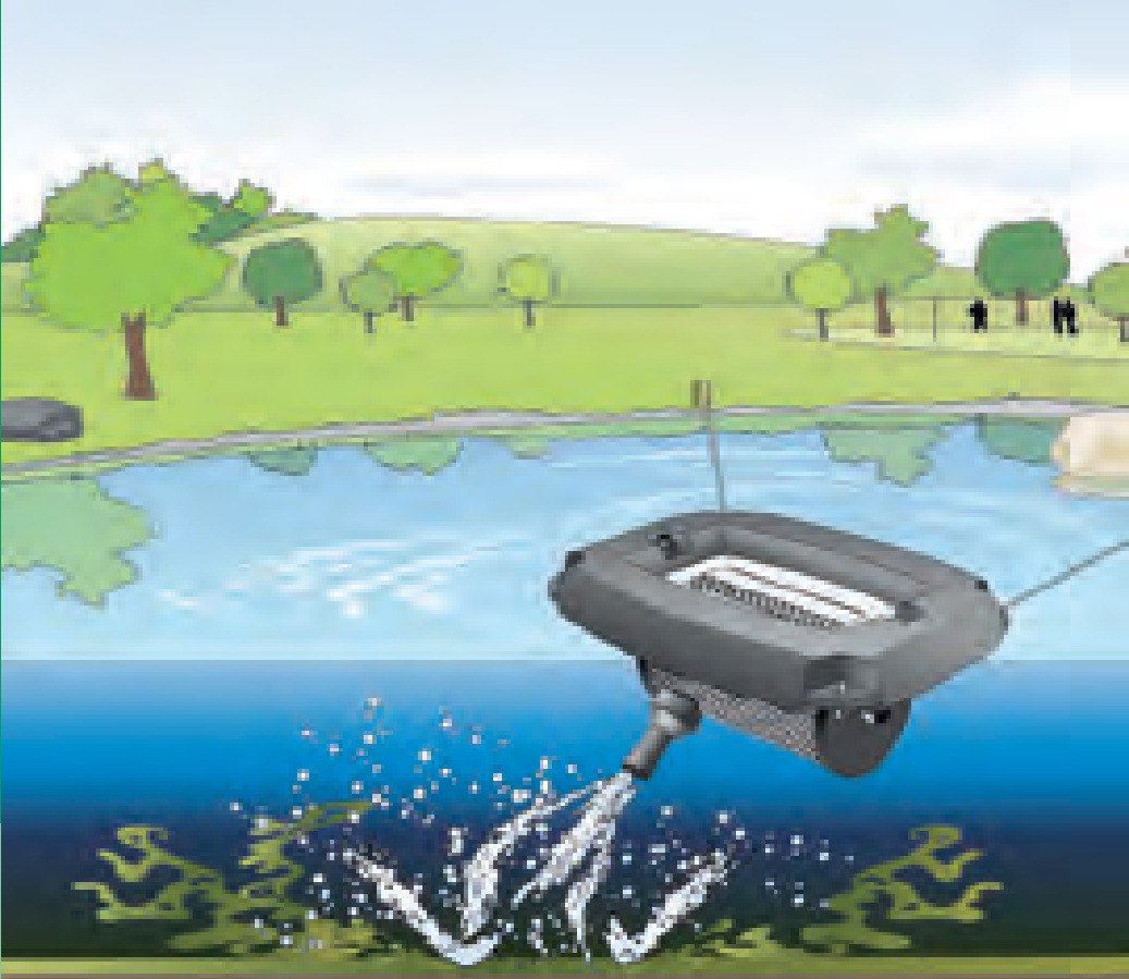
Schematic diagram: Pond aerator AquaAir 250 in use - distributes oxygen in the pond
