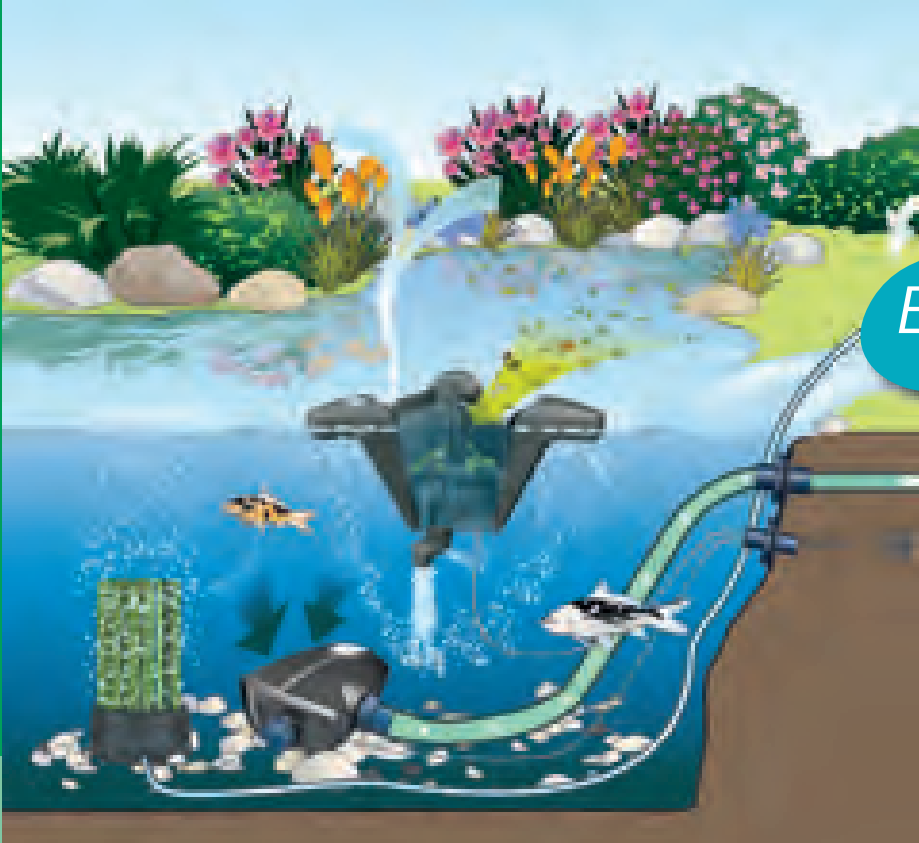
Schematic diagram: Interplay of the different components of the Clear Water System
