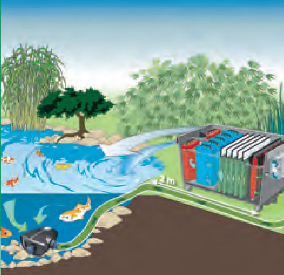
Schematic diagram: BioTec 30 in function with a filter and watercourse pump and a Bitron C
