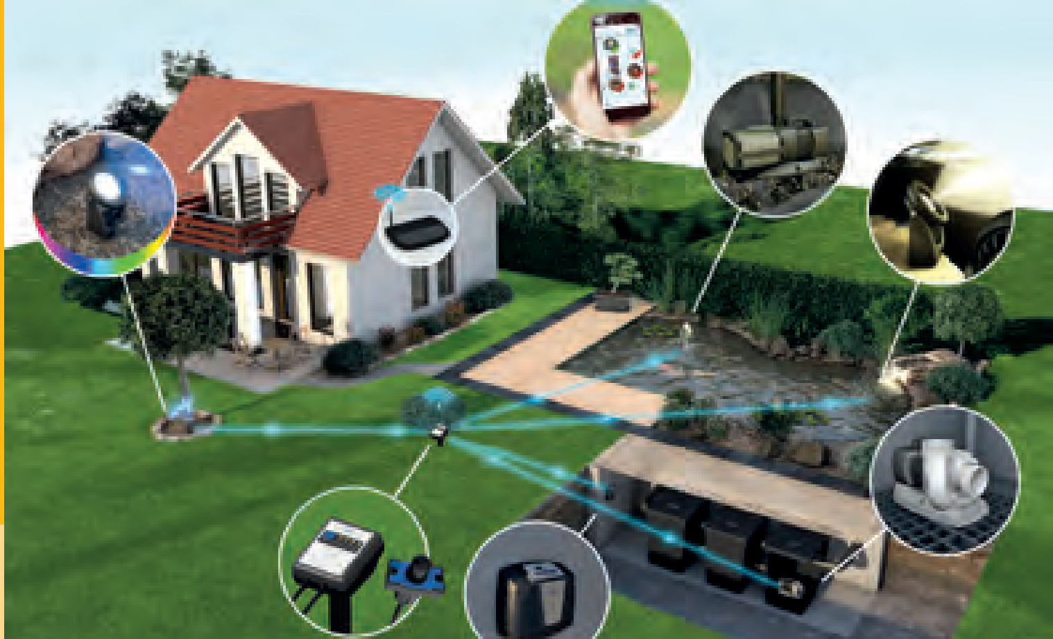
Schematic diagram: InScenio EGC Controller networked with router and EGC-capable OASE devices
