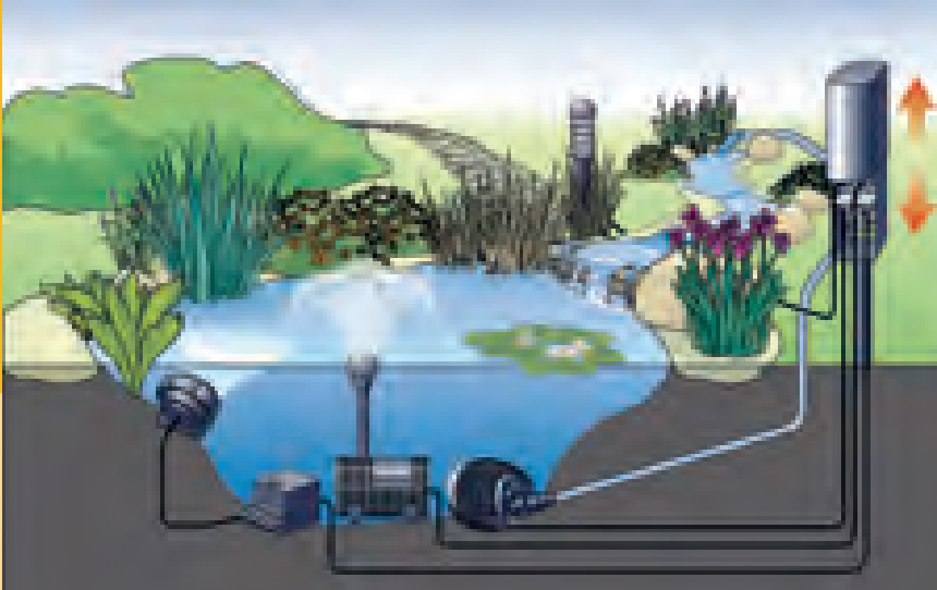
Schematic diagram: Connection possibilities with the OASE InScenio garden outlets
