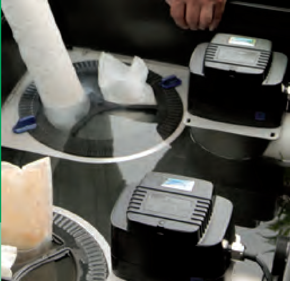
Bitron Gravity inserted in the Individual module of the ProfiClear Premium system
