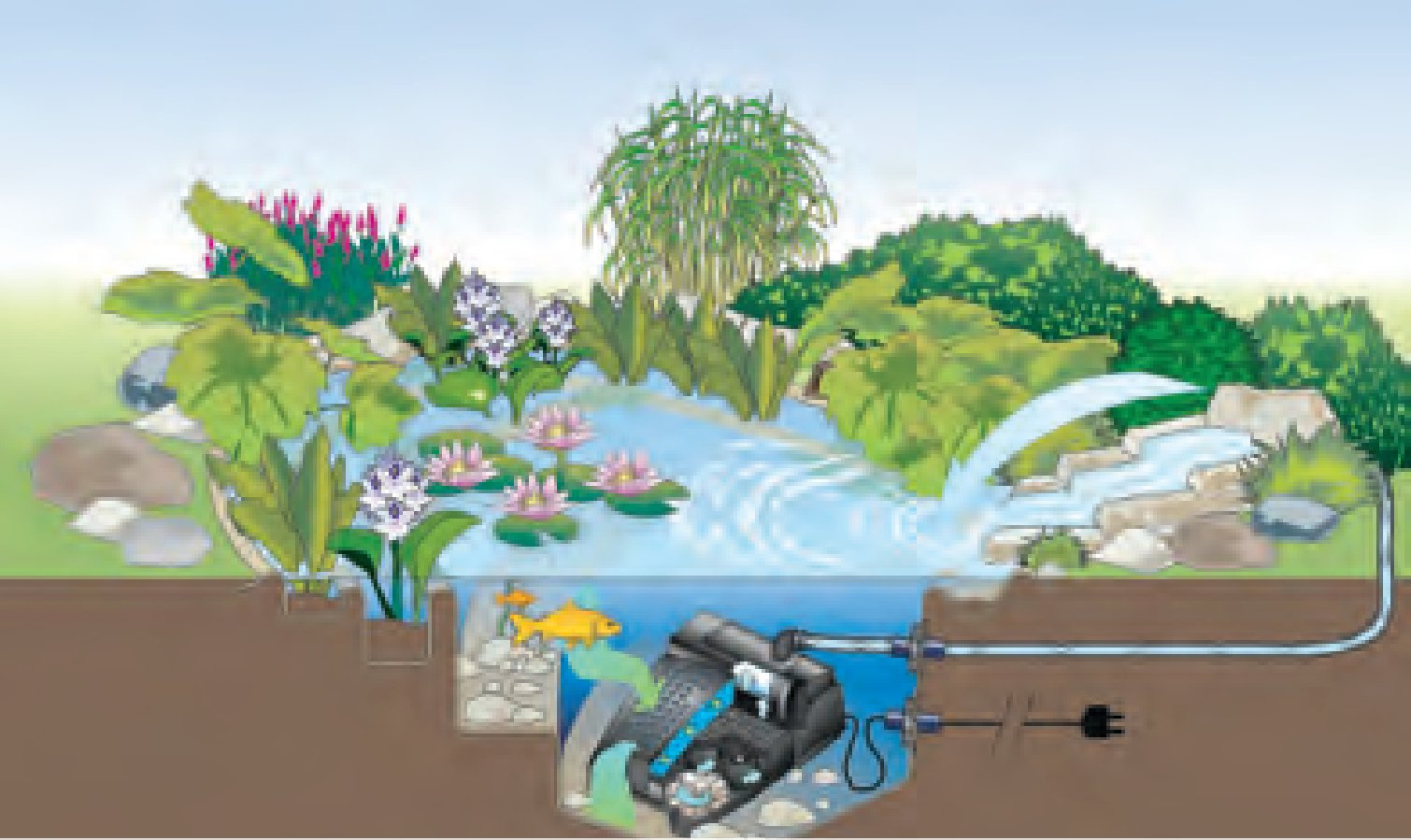
Schematic diagram: Underwater filter Filtral UVC (GB-Version) used in a pond pool
