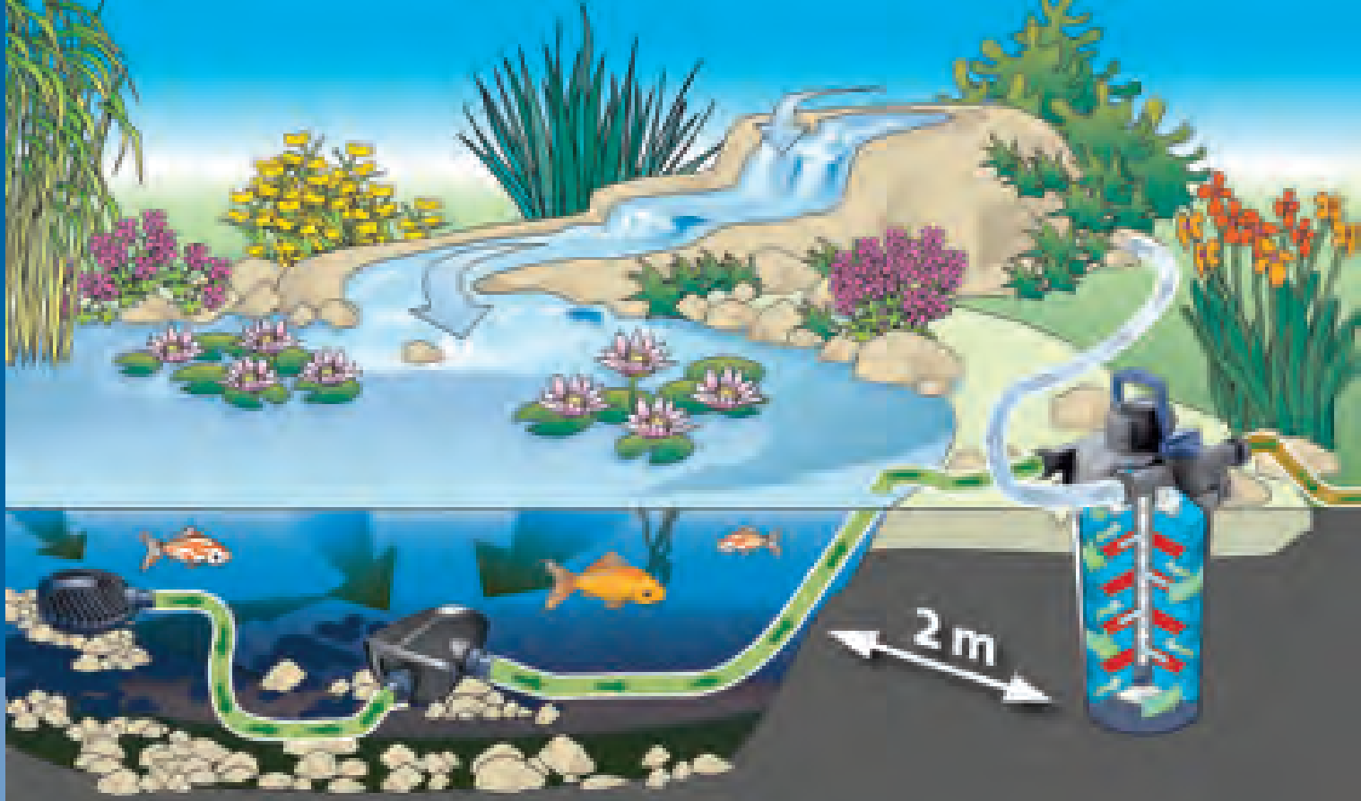
Schematic diagram: Pressure filter FiltoClear in combination with filter and watercourse pump
