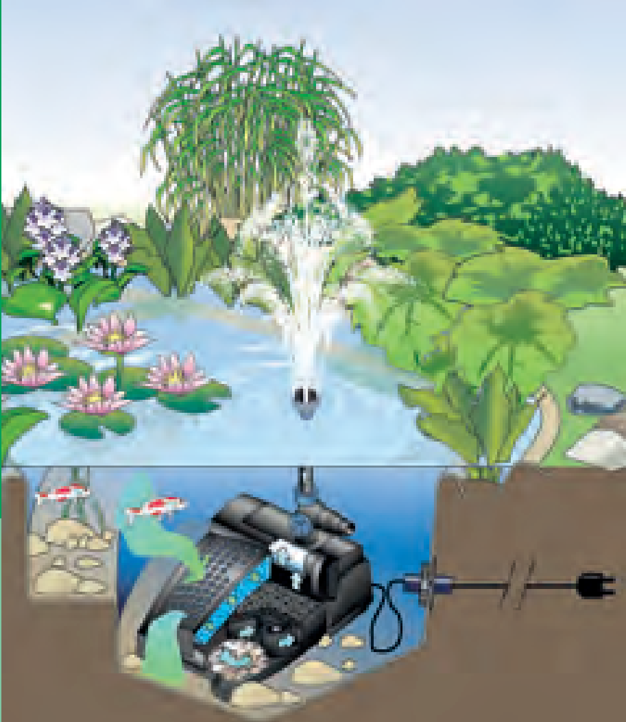
Schematic diagram: Underwater filter Filtral UVC inserted in a pond pool
