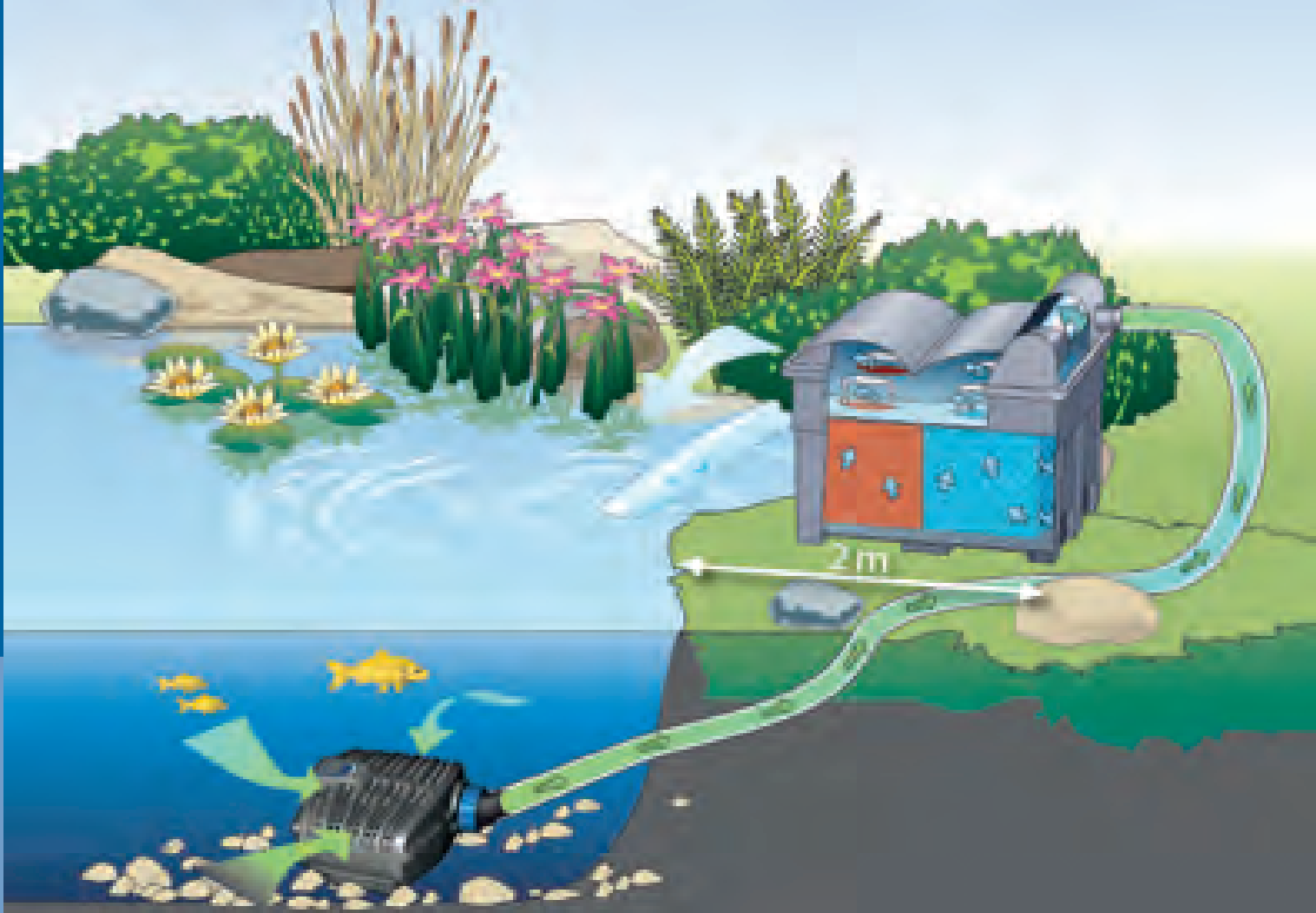
Schematic diagram: BioSmart UVC 16000 in combination with filter and watercourse pump AquaMax Eco Classic
