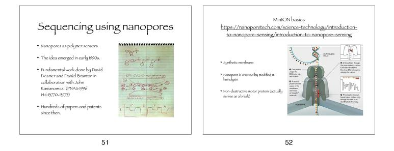
MinION basics https://nanoporetech.com/science-technology/introductionto-nanopore-sensing/introduction-to-nanopore-sensing • 512 channels (pores) per flow cell. (Isually about 90% are working. Read length: > 10 Kb (Phage \lambda DNA, 50 Kb) • Read speed: 8 bases to 20 bases/sec • Run time: max 48 hours • Error rate = 5-10 %
