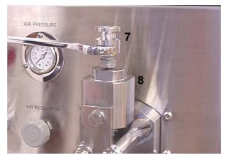
**Figure 7:** Removing an inlet fitting (7) from the inlet check valve (8). This inlet fitting is sanitary in design.
