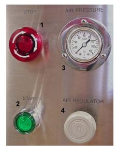
**Figure 2:** Close up view of the standard controls on the EmulsiFlex-C3 control box.
