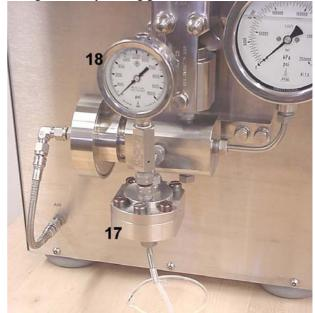
**Figure 4:** Filter/extruder assembly (17) and pressure gauge (18) mounted on an EmulsiFlex-C3.
