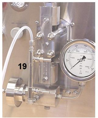
**Figure 5:** High efficiency heat exchanger (19) fitted to the outlet of the homogenizing valve.
