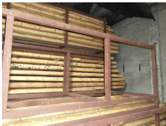
Figure 45: Kiln drying of bamboo, Colombia (Kaminski, 2016)
