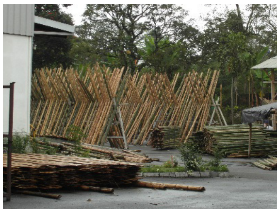
Figure 44: Air drying of bamboo outside, Colombia (Kaminski, 2016)
