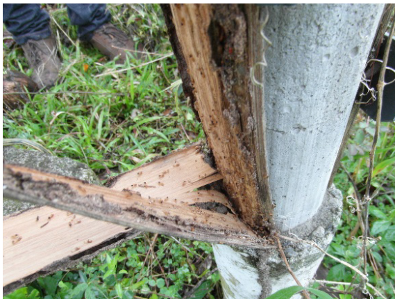
Figure 32: Termites attacking bamboo, Costa Rica. The termites are just visible as the translucent insects crawling on the inside of the bamboo (Kaminski, 2016)
