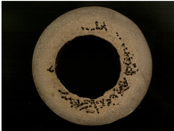
Figure 36: Cross-section through insect-damaged bamboo (Trujillo, 2014)
