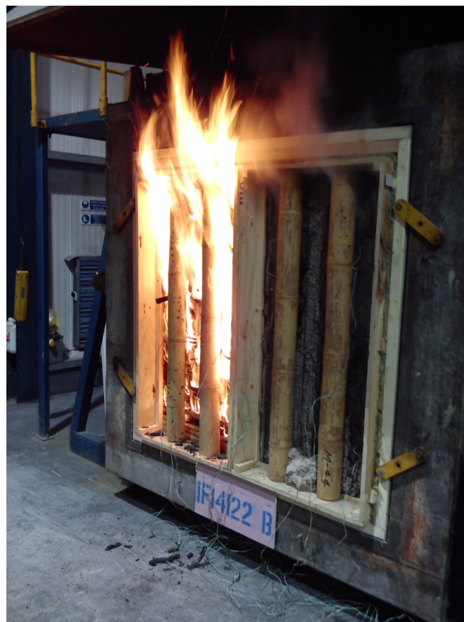
Figure 49: Fire tests on engineered bahareque at Trada (Webb, 2015)
