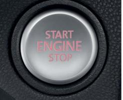
The Keyless entry system enables you to enter and exit your vehicle without taking the key out of your pocket. Once inside, as long as you have the key on you, the engine can be started without inserting the key in the ignition by simply pressing a button in the centre console. Optional on all models expect Beetle and Beetle Cabriolet.
