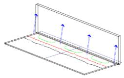
For wall mounted applications, a slight tilt out away from the wall creates a uniform well-lit path of egress. Traditional circular pattern optics require multiple iterations using complex angles to meet the NFPA 101 requirements of 1fc-average, 1fc-minimum, and 40:1 maximum-to-minimum uniformity.
