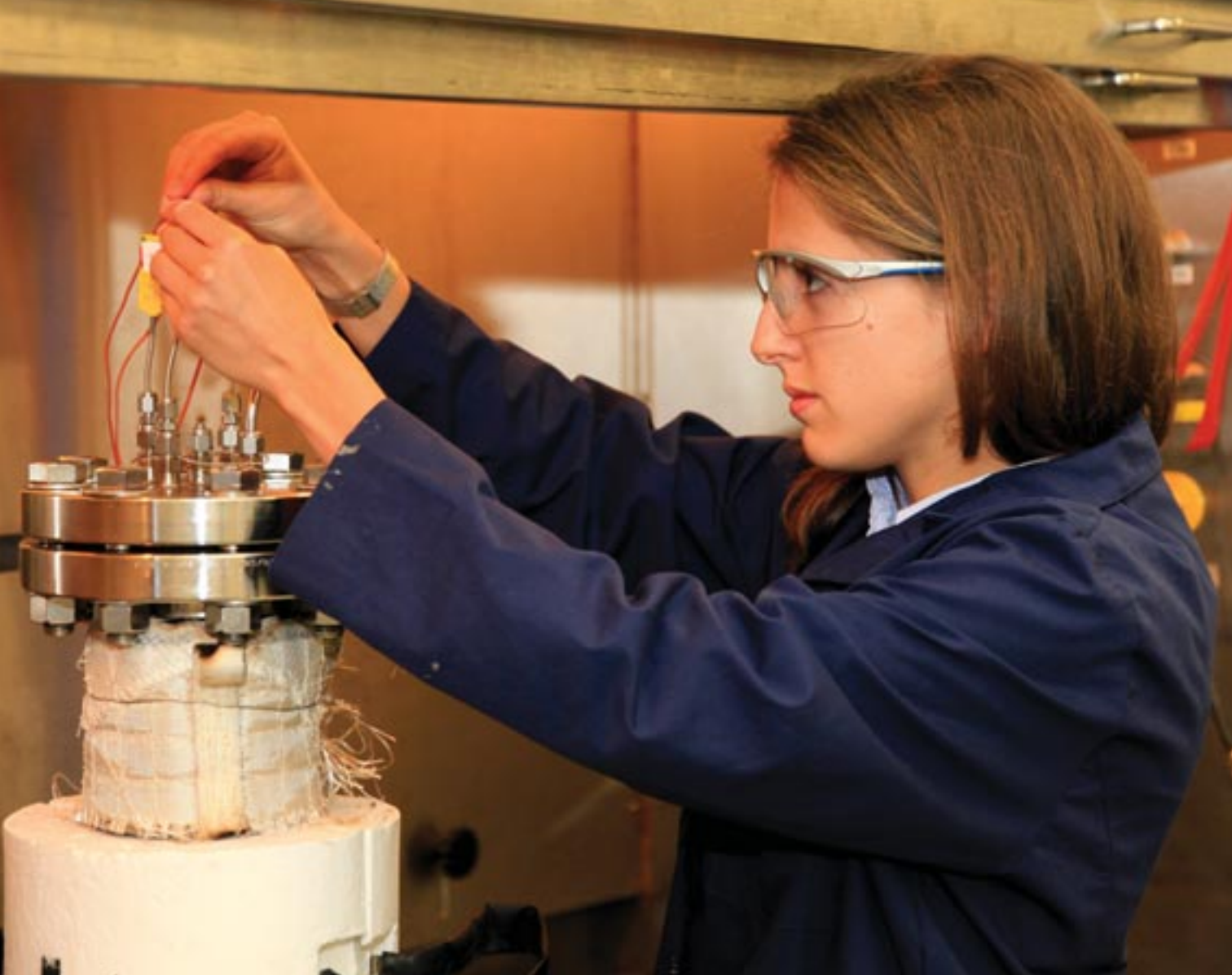
Kennedy Space Center chemical engineer Annie Meier adjusts the trash-to-gas reactor she is developing to recycle trash during deep space missions. Materials such as scraps, wrappers, packaging, and other garbage could be converted into methane gas, oxygen, and water. (NASA/Dan Casper)
