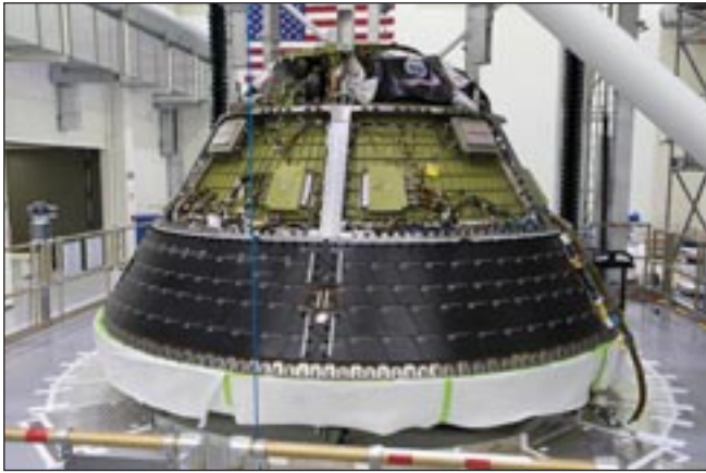
Heat shield back shell panels are prefitted on the Orion spacecraft inside the Neil Armstrong Operations and Checkout Building high bay. The back shell panels serve as the outer layer of the spacecraft and will protect it against the extreme temperatures of re-entry from deep space. (NASA/Kim Shiflett)
