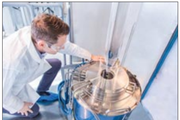
OFC 05 Horizontal OVD Cladding & OFC 08 Clad Sintering System
