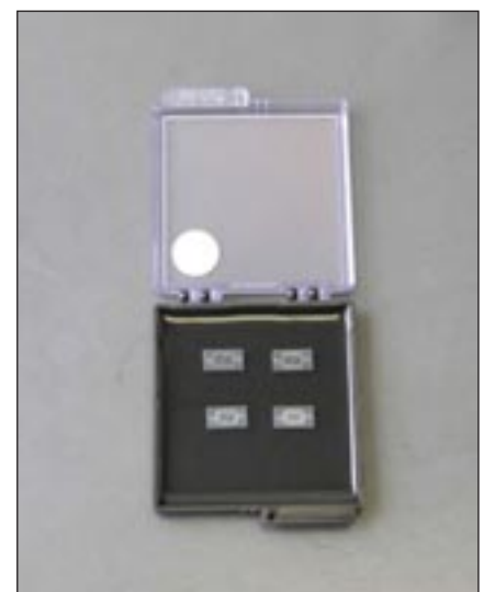
This figure shows four silicon-Pyrex wafers with 40-, 60-, 80-, and 100-mm length microchannels, respectively.
