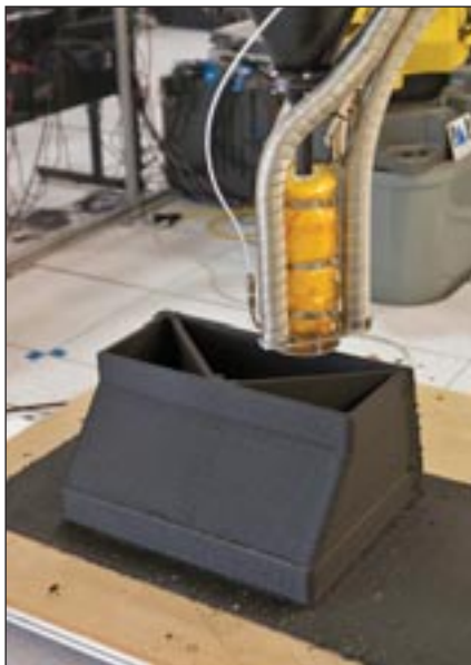
A Zero Launch Mass 3D printer is being tested at the Swamp Works at KSC. The printer can be used for construction projects on the Moon and Mars. It uses pellets made from simulated lunar regolith (dirt) and polymers, enabling astronauts to use resources at their destination instead of taking everything with them. (NASA/Glenn Benson)
