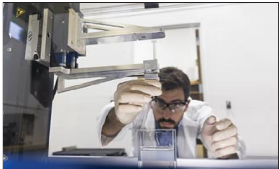
Silicone is 3D-printed into the micro-organogel support material. The printing nozzle follows a pre-defined trajectory, depositing liquid silicone in its wake. The liquid silicone is supported by the micro-organogel material during this printing process.
