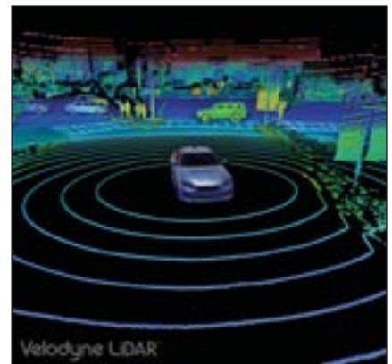
Figure 3. Velodyne's Surround View platform achieves a 360° view around the sensor by using a solid-state electronic lidar engine, which is essentially rotated on a spindle.
