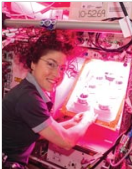
NASA astronaut Christina Koch initiates the Veg-PONDS-02 experiment on the International Space Station within Veggie by filling the upper reservoir. (NASA/David Saint-Jacques)
