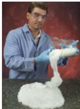
The Supergel system safely captures and disposes of radioactive elements in porous structures. The technology could be used in the event of an attack using a "dirty bomb" or other radioactive dispersal device.
