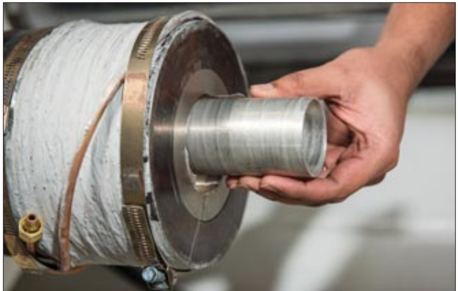
In ShAPE, a canister holding feedstock material is forced into a rotating die. Frictional heating is generated at the interface between the feedstock material and die, softening only the material being extruded and eliminating the need for external heat used in conventional extrusion.
