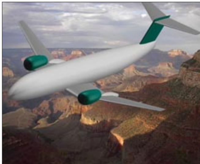
Noise is reduced because the engine nozzle is tangential to the wing upper surface and near the middle of the wing chord.
