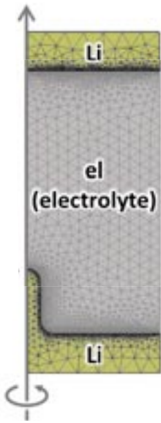
FIGURE 2. Mesh of the lithium-ion battery geometry.
