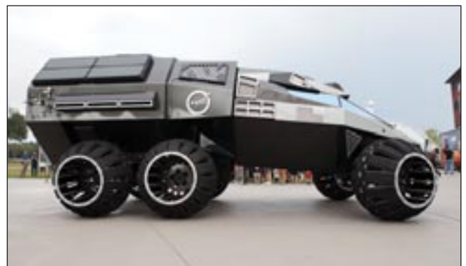
A Mars rover concept vehicle operates on an electric motor, powered by solar panels and a 700-volt battery. The rover separates in the middle with the front area designed for scouting and equipped with a radio and navigation provided by the Global Positioning System. The back section serves as a full laboratory that can disconnect for autonomous research. (NASA/Kim Shiflett)
