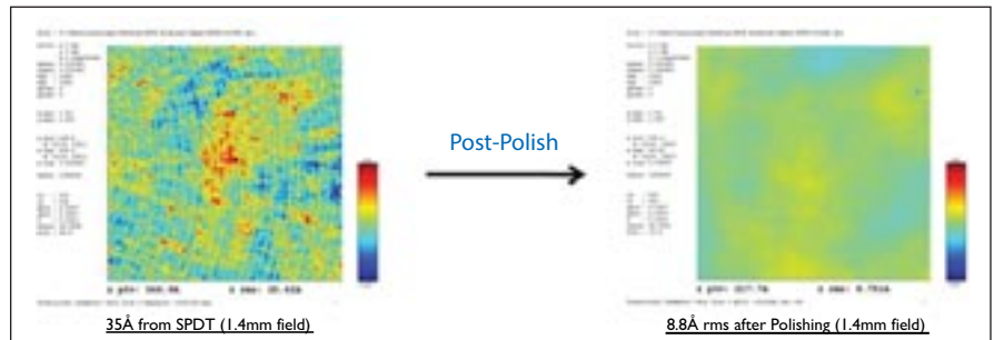
Figure 1. An important material advance is the ability to create optical quality surfaces on aluminum substrates, by deterministic polishing of surfaces created by SPDT.
