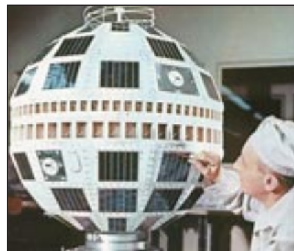
Telstar 1 — a 171-pound, 34.5-inch sphere with solar panels covered with sapphire cover plates — was placed in orbit on July 10, 1962.
