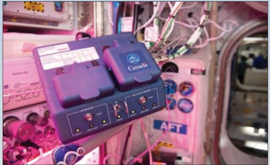
The Bio-Analyzer enables near-real-time, onboard analysis using biological samples such as blood, urine, saliva, sweat, and cell cultures. This diagnostic tool could help test specific countermeasures that are key to future exploration missions to the Moon, Mars, and beyond. (NASA)
