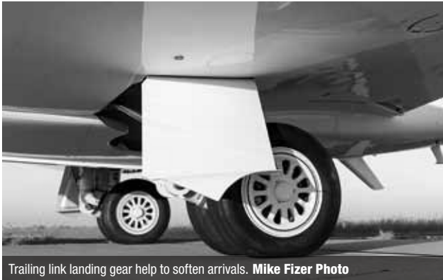
Trailing link landing gear help to soften arrivals. Mike Fizer Photo
