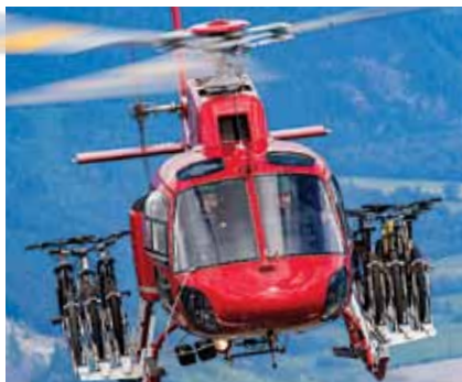
Newly certified bicycle racks for the Airbus Helicopters AS350/355 are getting a lot of attention from cyclists and heli-tourism companies around the world. Aero Design/Matthew Melsness Photo
