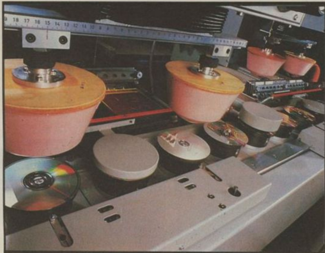
■ On the production line: CD 'sons' are used as stampers to produce thousands of CDs each day.
