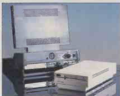
The printer port doubles as an interface for a 5.25in. disc drive.
