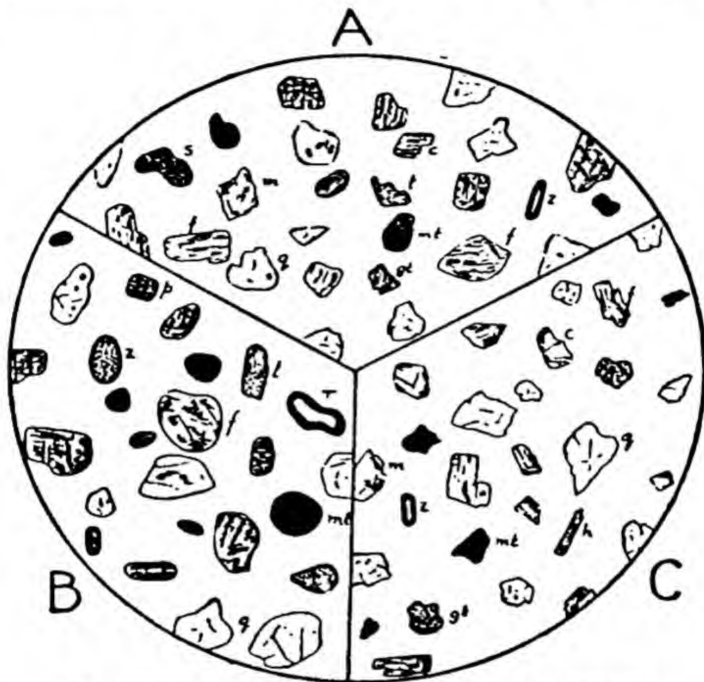
FIG. 54 — SHAPE AND ROUNDING OF SAND GRAINS.
