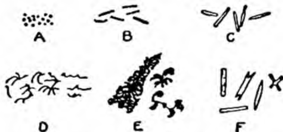
FIG. 35.—CRYSTALLITES AND MICROLITES. A, globulites; B, margarites; C, longulites; D, trichites; E, scopulites; F, microlites. Magnification about 200 diameters.
