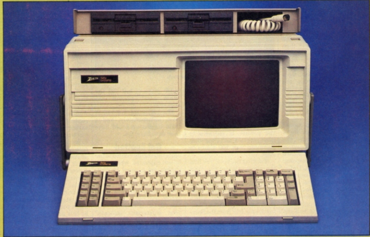
The Zenith Z160 is more of a movable desk top machine than a portable. Note the brown screen which is comfortable to use for long periods.
