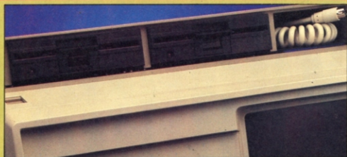
The disk drives 'pop-up' from the top of the machine and are supported by two 'bed springs'.
