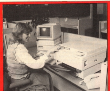
SPEED OF LIGHT — All right, we know it is expensive at around £3,000 but wouldn't you just like to own a laser printer like this. The EPS LaserJet prints at eight A4 pages per minute, can mix up to four typefaces on a single page and has a print resolution of 300 dots per inch. Prices of laser printers are starting to tumble, so who knows, it may not be long before you can buy one for £1,000. Meanwhile carry on with your dot matrix and dream.
