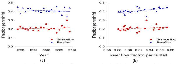
Figure 5. Fraction of surface flow and base flow rates against the rainfall during the 20 years of observation (a) against the river flow fraction (river discharge) per rainfall (b)
