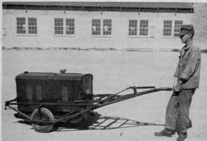
One man can pull the generator.
