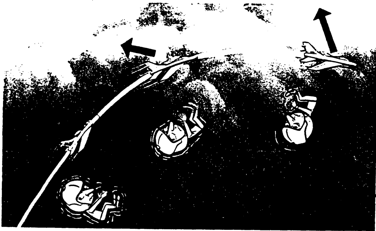
Figure 19. The inversion illusion. Centrifugal and tangential inertial forces during a level-off combined with the force of gravity to produce a resultant gravito-inertial force that rotates backward and upward with respect to the pilot, causing him to perceive that he is suddenly upside down. Turbulent weather can produce additional inertial forces that contribute to the illusion. (Adapted from Martin and Jones.) 10
