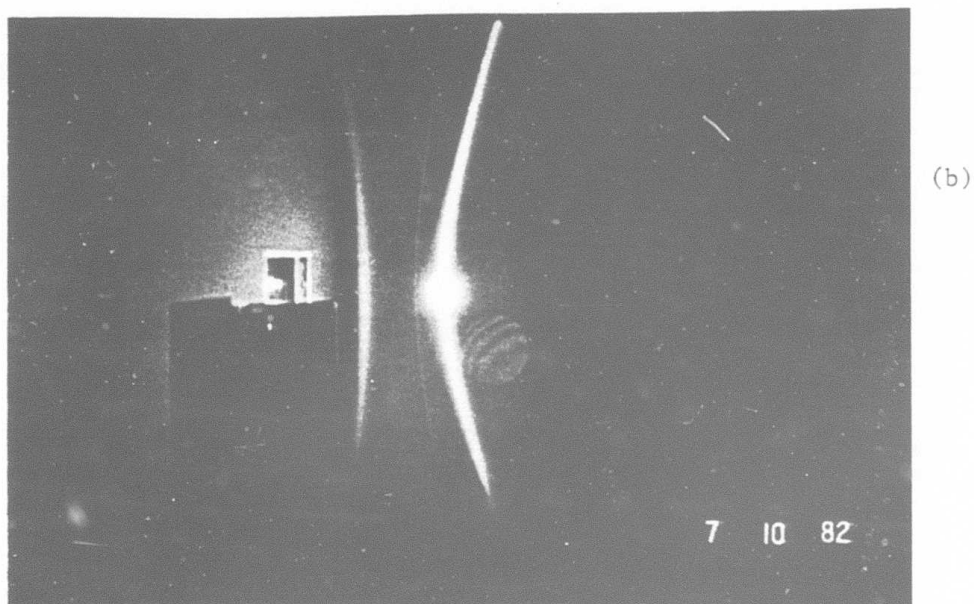
Figure 3.15. Photographs of the illumination of a screen by the light reflected from the films at resonance. The electromagnetic wave is scattered mainly in the dielectric layer of Fig. 3.14 and emerges as part of a cone of light.
