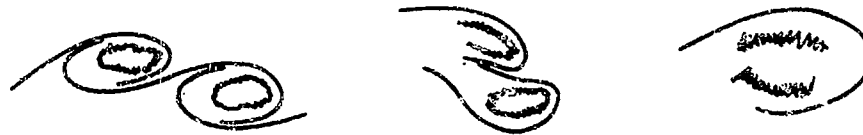
Figure 1 Schematic Diagram Showing Vortex Development and Pairing.
