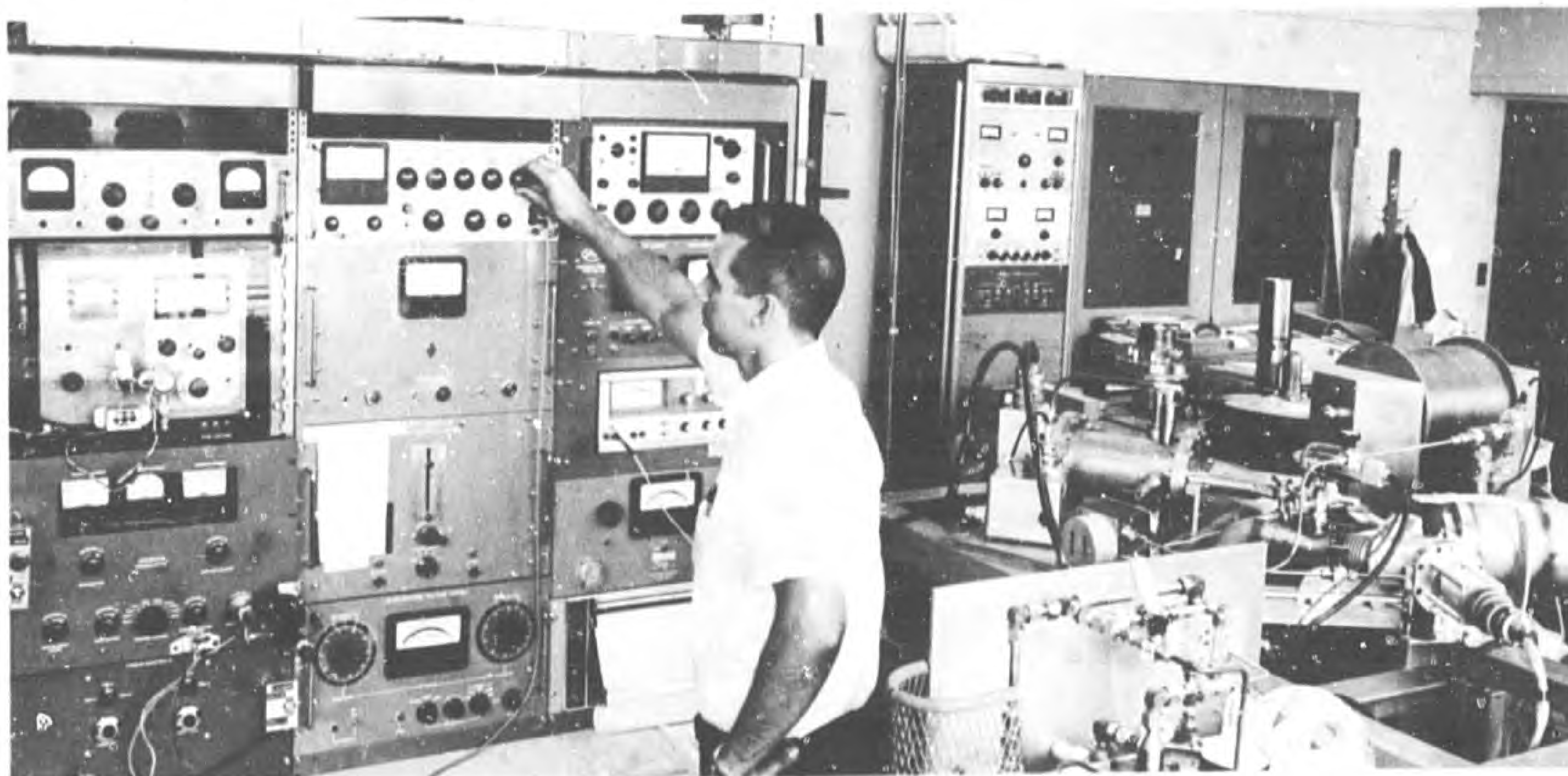
Figure 3. Mass spectrometer used to measure the currents of the reactant and product ions as a function of the kinetic energy of the reactant ions.
