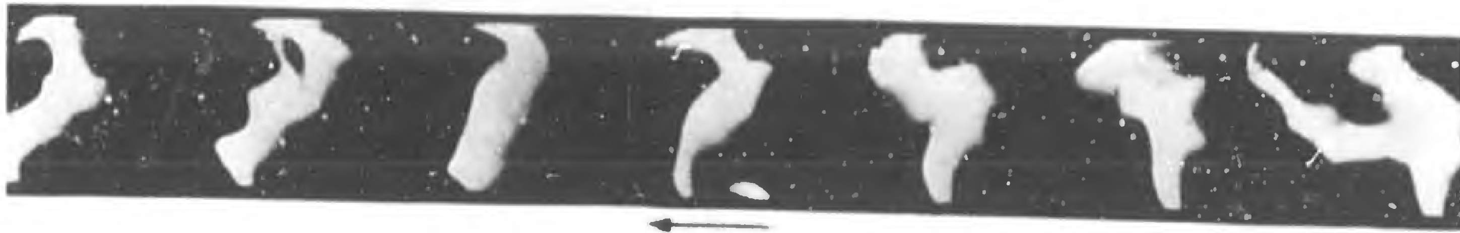
HIGH-SPEED PHOTOGRAPHS OF ARC MOTION ALONG RAIL ELECTRODES (26,000 frames/sec.)
