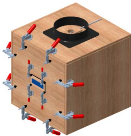
Figure 2-13. Pressure Chamber: Three dimensional representation of the pressure chamber holding the plywood sample (left) and actual pressure chamber used for tape leakage tests (right).
