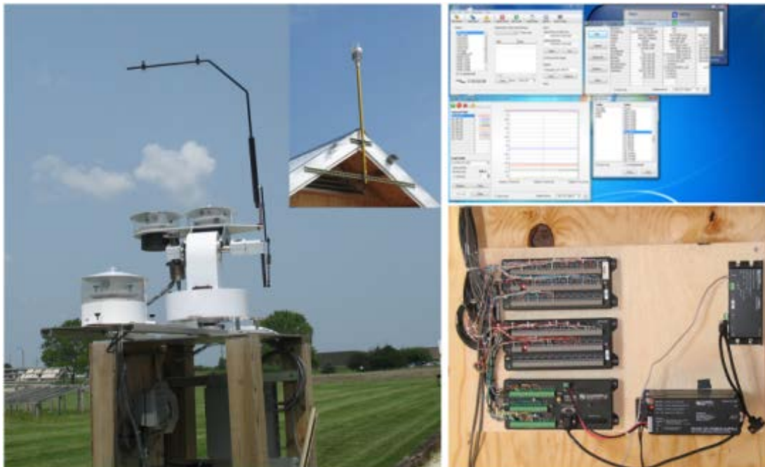
Figure 4-1. Weather station and data acquisition system with remote access capability.
