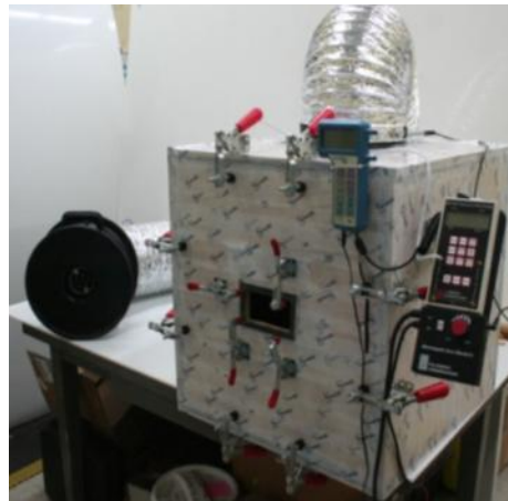
Figure 2-13. Pressure Chamber: Three dimensional representation of the pressure chamber holding the plywood sample (left) and actual pressure chamber used for tape leakage tests (right).
