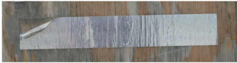
Figure 2-19. Tape D after Outdoor Exposure: Tape D after 8 months of outdoor exposure in the horizontal SW (right) locations.
