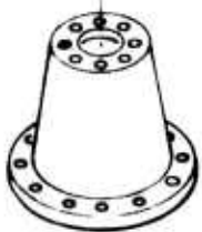
B-5 CLAMSHELL ROTOR HEAD WT - 1,24 LB COST - $31,250
