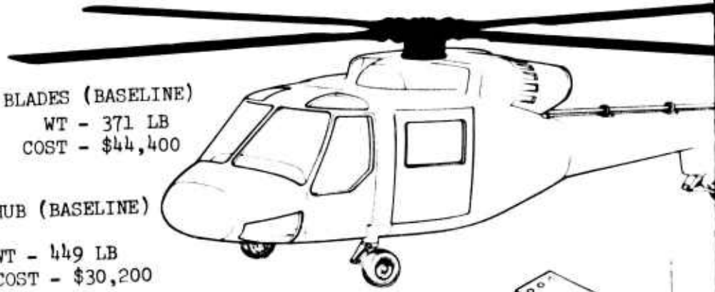
B-1 PADDLE TIP ROTOR BLADE WT - 334 TO 408 LB COST - $29,300 TO $32,000
