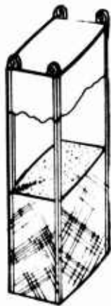
A-15 MOLDED COMPOSITE BOX STRUCTURE, PYLON
