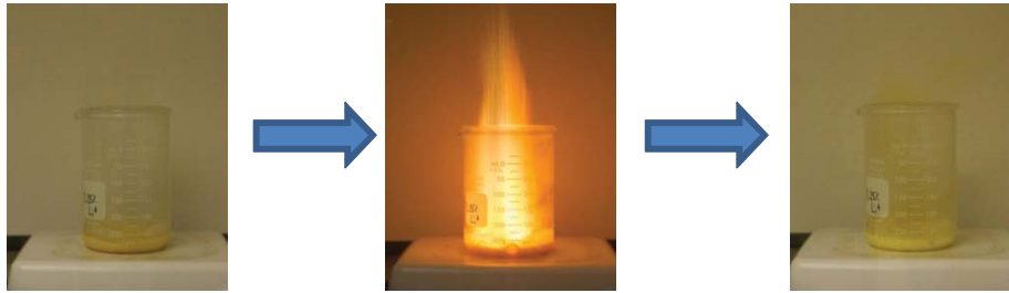
Fig. 4. Example of synthesis of MgO doped with a lanthanide (Ln) using the Solution Combustion Synthesis technique.
