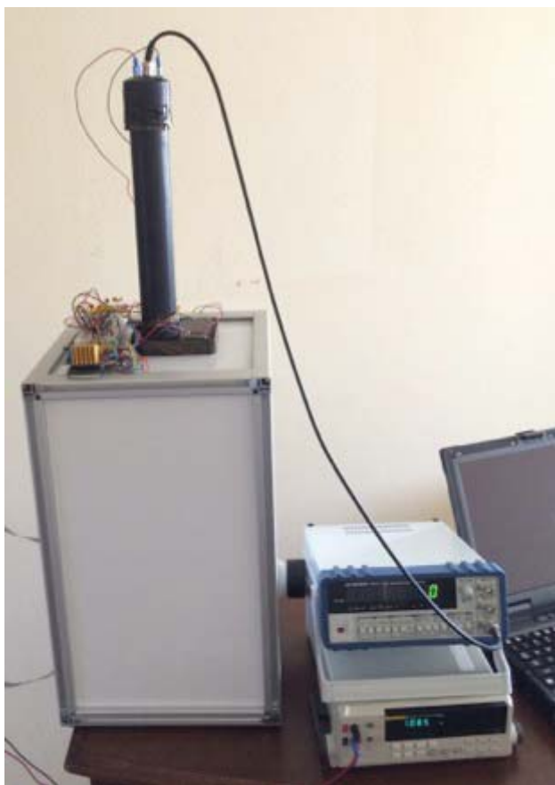
Fig. 152. Exterior of the portable TL readout system. From left to right: light-tight hotplate enclosure, with black tubular PMT mount and motorized shutter system on top; frequency counter and hotplate temperature sensor instruments; and data collection laptop.
