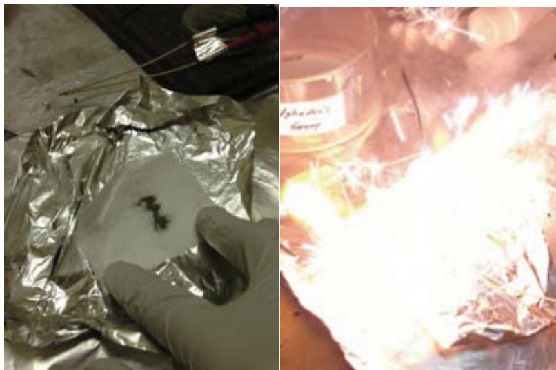
Fig. 108. A piece of flash paper with titanium powder being prepared (left) and in mid-burn (right). While not shown here, in runs testing TL materials, the TL powder is mixed into the titanium powder or placed wherever desired, and recovered from the container in which the burn takes place. Generally, very little unburned nitrocellulose or titanium powder remains.
