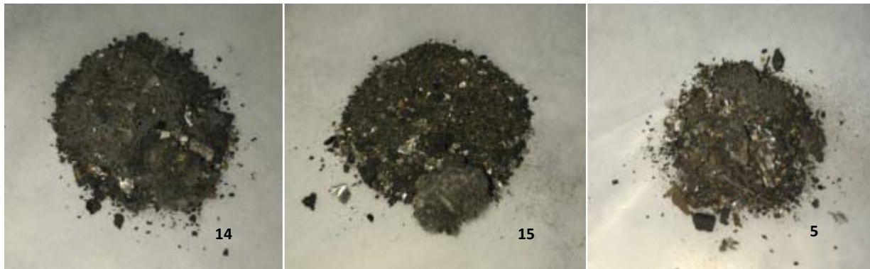
Fig. 146. Photographs of the post-detonation TLD-100 and debris returned from Indian Head. From left to right: "shot 14 LPBX", "shot 15 LPBX", and "shot 5 HPBX".
